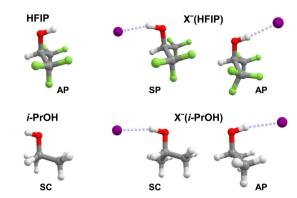
Fig. 2 Minimum-energy structures of HFIP, i-PrOH, X<sup>-</sup>(HFIP) and X<sup>-</sup>(i-PrOH). The lowest energy conformer for the neutral molecules and the two lowest energy isomers for the anion complexes are shown. See Table 2 for relative energies and geometric parameters.
