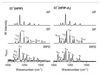
Fig. 3 Unscaled harmonic MP2/aug-cc-pVTZ IR spectra of the AP (top panel) and the SP isomer (see Fig. 2 for geometries) of Cl<sup>-</sup>(HFIP) (left) and Cl<sup>-</sup>(HFIP- $d_1$ ) (right) compared to the IRPD spectrum of the corresponding D<sub>2</sub>-tagged complex. See Table 3 for band positions, harmonic vibrational frequencies and assignments. The harmonic spectra were convoluted using a Gaussian line-shape function with a full width at half maximum (FWHM) of 8 cm<sup>-1</sup>.
