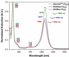
Fig. 6 Experimental UV/VIS/NIR spectra of [Ni(cAAC<sup>Me</sup>-CS<sub>2</sub>)<sub>2</sub>] (3a, green), [Ni(IDipp-CS<sub>2</sub>)<sub>2</sub>] (3b, blue) and [Ni(IMes-CS<sub>2</sub>)<sub>2</sub>] (3c, red) in TD-DFT (PBE0-D3BJ//def2-TZVPP(Ni)/def2-TZVP(C,H,N,S)/COSMO(benzene)) calculated absorption maxima  $\lambda_{calc}$ for the NIR absorption ( $\omega_1$ ).
