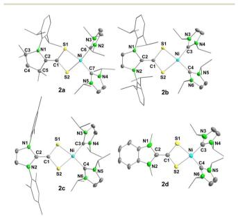
Fig. 1 Molecular structures of  $[Ni(|^iPr)_2(cAAC^{Me}-CS_2)]$  (2a, top left),  $[Ni(|^iPr)_2(IDipp-CS_2)]$  (2b, top right),  $[Ni(|^iPr)_2(IMes-CS_2)]$  (2c, bottom left), and  $[Ni(|^iPr)_2(BIMe-CS_2)]$  (2d, bottom right) in the solid-state (ellipsoids set at the 50% probability level). The hydrogen atoms were omitted for clarity. Selected bond lengths [Å] and angles [°] are provided within Table 1 or in the captions of Fig. S72–S75 of the ESI.‡
