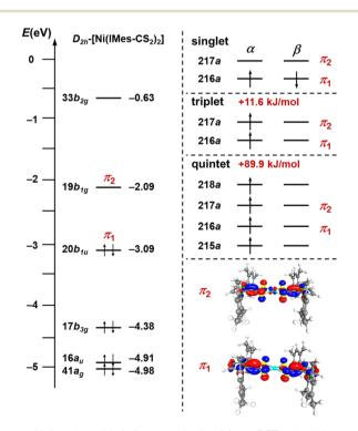
Fig. 4 Molecular orbital diagram obtained from DFT calculations on geometry-optimized,  $D_{2h}$ -symmetric [Ni(IMes-CS<sub>2</sub>)<sub>2</sub>] (**3c**) at the B3-LYP//def2-TZVP(Ni)/def2-SVP(C,H,N,S) level of theory and the relative energies of the singlet, triplet, and quintet state of this complex. The MOs and an overview of the changes in selected geometric parameters of **3c** in different electronic states are provided in Fig. S3 and S4 of the ESI.‡
