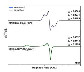
Fig. 9 βX-band EPR spectra of K[Ni(cAAC<sup>Me</sup>-CS<sub>2</sub>)<sub>2</sub>] (4a<sup>K</sup>, bottom, green) and K[Ni(IDipp-CS<sub>2</sub>)<sub>2</sub>] ( $4b^{K}$ , top, blue) at 70 K with normalized xand y-axes (exact values are provided in Fig. S32-S34 of the ESI;‡ resonances are detected at ca. 310-340 mT; black lines: simulated spectra; regular, colored lines: experimental spectra)
