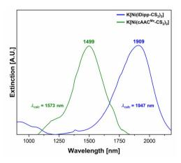
Fig. 10 Experimental UV/VIS/NIR absorption spectra of K[Ni(cAAC<sup>Me</sup>- $(CS_2)_2$  (4a<sup>K</sup>, green) and K[Ni(IDipp- $(CS_2)_2$ ) (4b<sup>K</sup>, blue) in THF in the NIR TD-DFT (PBE0-D3BJ//def2-TZVPP(Ni)/def2-TZVP(C,H,N,S)/COSMO(THF)) calculated absorption maxima  $\lambda_{calc}$
