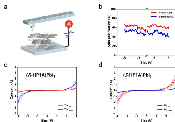
Fig. 5 (a) Schematic representation of the mCP-AFM measurements. (b) Average values of spin polarization in  $(R\text{-HP1A})\text{PbI}_3$  (red) and  $(S\text{-HP1A})\text{PbI}_3$  (blue). (c and d) Room-temperature mCP-AFM measurements for  $(R/S\text{-HP1A})\text{PbI}_3$ . The shaded region around the lines marks the standard deviation for the average results.
