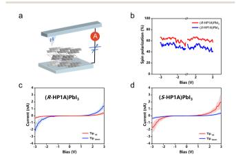
Fig. 5 (a) Schematic representation of the mCP-AFM measurements. (b) Average values of spin polarization in (R-HP1A)Pbl<sub>3</sub> (red) and (S-HP1A)Pbl<sub>3</sub> (blue). (c and d) Room-temperature mCP-AFM measurements for (R/S-HP1A)Pbl<sub>3</sub>. The shaded region around the lines marks the standard deviation for the average results.
