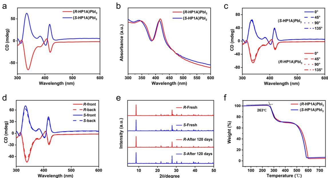
Fig. 2 (a and b) CD (a) and UV-vis absorption (b) spectra of  $(R/S\text{-HP1A})\text{PbI}_3$  films. (c and d) Angle-dependent (c) and direction-dependent (d) CD spectra of  $(R/S\text{-HP1A})\text{PbI}_3$  films. (e) XRD patterns of  $(R/S\text{-HP1A})\text{PbI}_3$  single crystals before and after 120 days. (f) TGA of  $(R/S\text{-HP1A})\text{PbI}_3$ .
