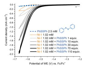
Fig. 4 Cyclic voltammogram (CV) of diphenyl disulfide (PhSSPh, 2.5 mM, blue dashed) and of Ni-1[ClO<sub>4</sub>] (1.02 mM, orange dotted) in the absence and presence of diphenyl disulfide (1, 10, 30, 70, 110 equiv., gray and black solid) at 0.1 V s<sup>-1</sup> in CH<sub>3</sub>CN containing TBAPF<sub>6</sub> (0.1 M). CV scans were initiated at -1.16 V vs. Fc/Fc<sup>+</sup>.
