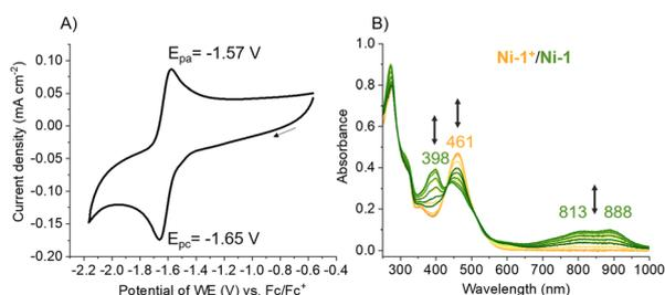
Fig. 3 (A) Cyclic voltammogram of  $Ni-1^+$  (1.5 mM) recorded at  $0.1$  V  $s^{-1}$  in  $CH_3CN$  containing  $TBAPF_6$  (0.1 M). (B) UV/vis-SEC of  $Ni-1^+$  (2.65 mM) recorded in  $CH_3CN$  containing  $TBAPF_6$  (0.6 M).  $Ni-1^+$  contains a Ni(II)-ion whereas  $Ni-1$  contains a Ni(I)-ion.
