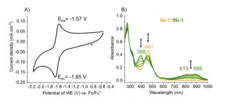
Fig. 3 (A) Cyclic voltammogram of Ni-1<sup>+</sup> (1.5 mM) recorded at 0.1 V s<sup>-1</sup> in CH<sub>3</sub>CN containing TBAPF<sub>6</sub> (0.1 M). (B) UV/vis-SEC of Ni-1<sup>+</sup> (2.65 mM) recorded in CH<sub>3</sub>CN containing TBAPF<sub>6</sub> (0.6 M). Ni-1<sup>+</sup> contains a Ni(II)-ion whereas Ni-1 contains a Ni(I)-ion.
