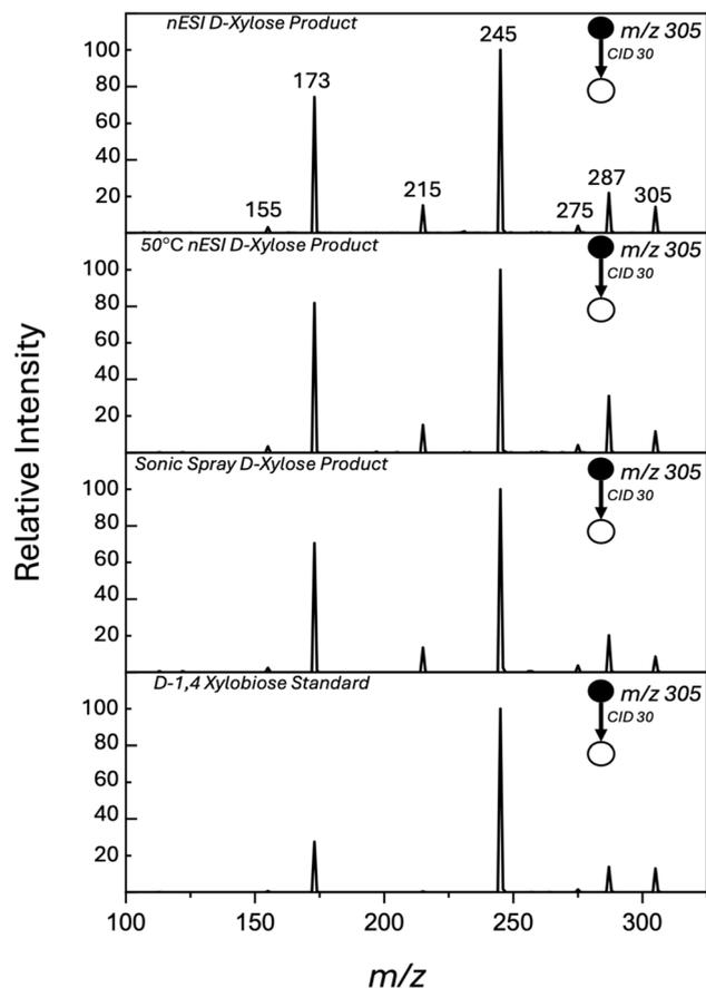
Fig. 2 MS/MS of ions  $m/z$  305 formed from 10 mM aqueous xylose solution using typical nESI conditions, mass-selected in an ion trap and fragmented by collision-induced dissociation (CID 30, manufacturers unit) (Top panel); compared to 50 °C capillary nESI (2nd panel); using sonic spray instead of nESI (3rd panel); compared to ions generated from authentic pentose disaccharide 1,4-D-xylobiose (bottom panel).
