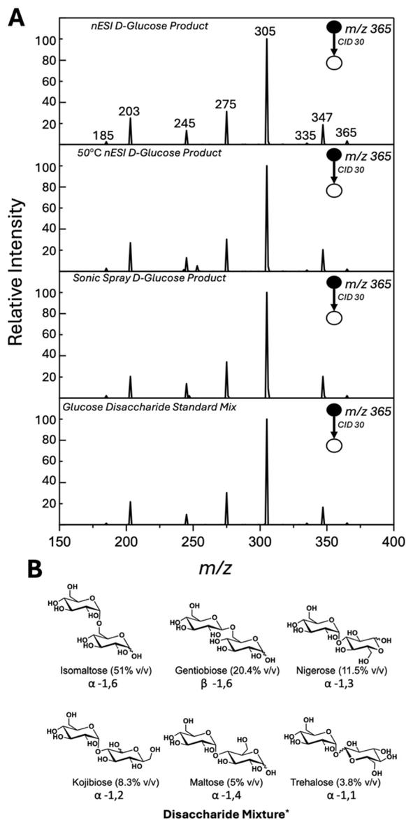
Fig. 3 (A) MS/MS of ions of  $m/z$  365 generated by nESI or sonic spray of glucose, mass selected in an ion trap and fragmented at CID 30 (manufacturers unit). (Top) Typical nESI conditions; (2nd panel) nESI with 50 °C inlet capillary; (3rd panel) sonic spray ionization; (Bottom) for disaccharide mixture. (B) Structures and volume fractions of disaccharides used in the disaccharide mixture. \*Disaccharide standard mixture based on ref. 80.
