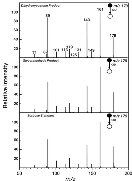
Fig. 1 Q-ToF tandem mass spectra of ions  $m/z$  179 formed from various compounds. (Top) MS/MS fragmentation of  $m/z$  179 ions from dihydroxyacetone. (Middle) MS/MS fragmentation of  $m/z$  179 ions from glyceraldehyde. (Bottom) MS/MS fragmentation of the  $m/z$  179 ions generated from authentic sorbose.
