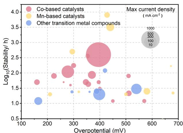
Fig. 8 Benchmarking of noble-metal-free OER electrocatalysts tested in acidic media. Overpotentials and stability of the catalysts at a current density of 10 mA cm<sup>-2</sup>. See detailed information in Table 1 for noble-metal-free catalysts.
