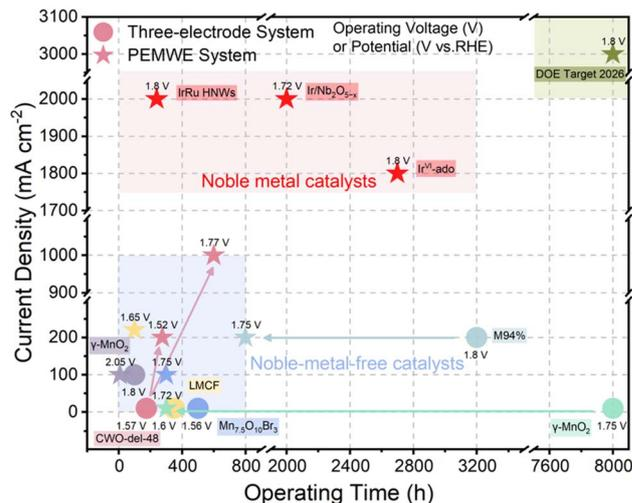
Fig. 9 PEMWE and three-electrode electrochemical cell performance comparison of reported non-noble metal OER catalysts. Representative Ir-based catalysts and DOE target 2026 are given for comparison.
