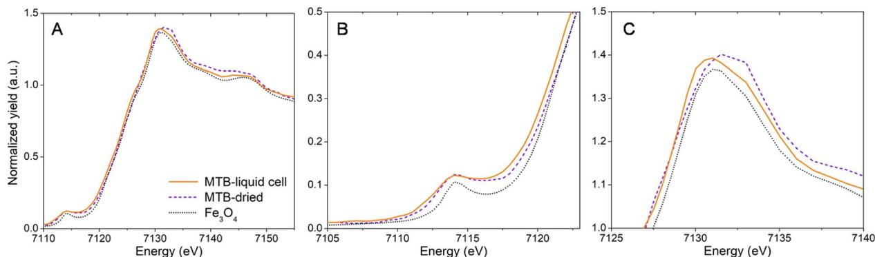
Fig. 2 (A) Fe K-edge X-ray absorption near-edge structure (XANES) spectra of MSR-1 bacteria under hydrated conditions (liquid cell) and dried conditions with a magnetite ( $\text{Fe}_3\text{O}_4$ ) reference. Zoomed in regions for (B) pre-edge (promotion of 1s electrons to unoccupied 3d valence levels) and (C) white-line (promotion of 1s electrons to unoccupied 4p valence levels) features.
