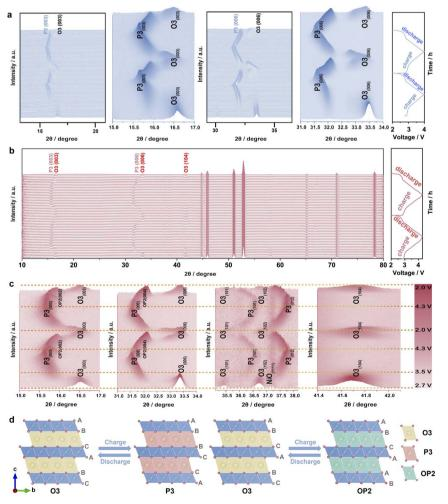
Fig. 4 Phase transition analysis of the NaNCMMT electrode during cycling. (a) In situ XRD patterns and 3D contour plots of characteristic peaks during the first two charge/discharge cycles at 0.1C in 2.0-4.0 V. (b) In situ XRD patterns for the first two charge/discharge cycles at 0.1C in 2.0-4.3 V. (c) 3D contour plots of diffraction peaks at 0.1C in 2.0-4.3 V. (d) Schematic illustration of structural changes during Na<sup>+</sup> extraction/insertion in 2.0-4.3 V.
