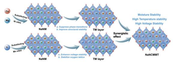
Scheme 1 Synergistic effects of Cu/Mg substitution for Ni and Ti substitution for Mn in NaNCMMT cathode.
