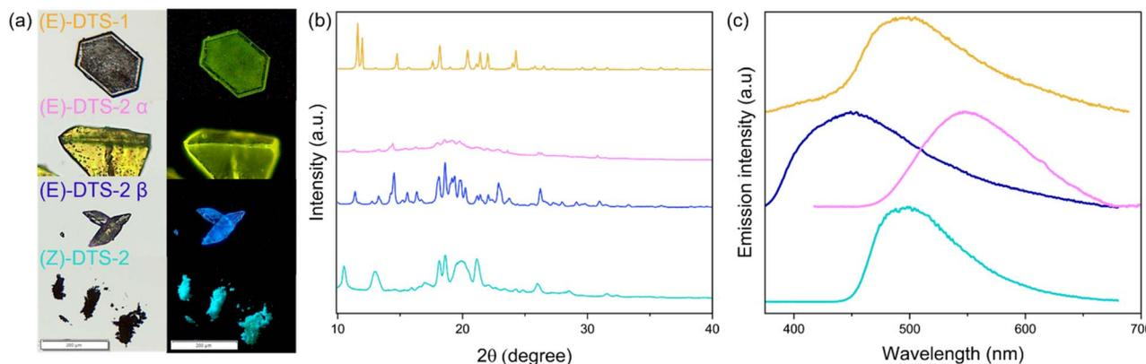
Fig. 8 (a) Photoluminescence spectra of crystalline powder of (*E*)-DTS-1 (yellow), (*E*)-DTS-2 in  $\alpha$  powder (pink),  $\beta$  powder (blue) and (*Z*)-DTS-2 (cyan). (b) XRD powder diffraction patterns for (*E*)-DTS-1 (yellow), (*E*)-DTS-2 in  $\alpha$  (blue) and  $\beta$  (pink) and (*Z*)-DTS-2 (cyan). (c) Optical microscope images of (*E*)-DTS-1 (yellow), (*E*)-DTS-2 in  $\alpha$  (blue) and  $\beta$  (pink) powder and (*Z*)-DTS-2 (cyan) under white light (left) and UV-light (right).
