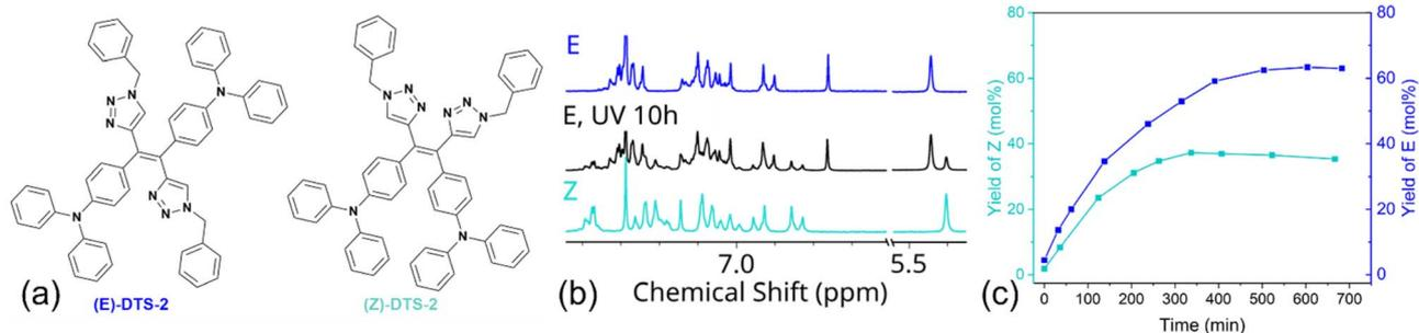
Fig. 5 (a) Structure of the isolated diastereoisomers of DTS-2 (b) partial <sup>1</sup>H NMR spectra of (*E*)-DTS-2 (blue), of irradiated (*E*)-DTS-2 (black) and (*Z*)-DTS-2 (cyan). (c) Isomerization yield of the initially pure (*E*) (blue) and (*Z*) (cyan) in CD<sub>2</sub>Cl<sub>2</sub> (10<sup>−3</sup> M) upon photoirradiation at 365 nm (4.7 mW cm<sup>−2</sup>) determined by NMR.
