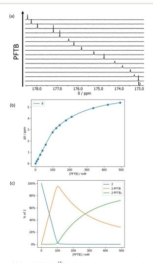
Fig. 8 (a) Partial 176 MHz  $^{13}$ C NMR spectra for titration of perfluorotert-butanol into 2 (92 mM) in n-octane at 298 K. (b) Best fit of the NMR data to a 1:2 binding isotherm ( $K_1 > 10^3 \text{ M}^{-1}$  and  $K_2 = 7 \text{ M}^{-1}$ ). (c) Speciation as a function of PFTB concentration.<sup>34</sup>
