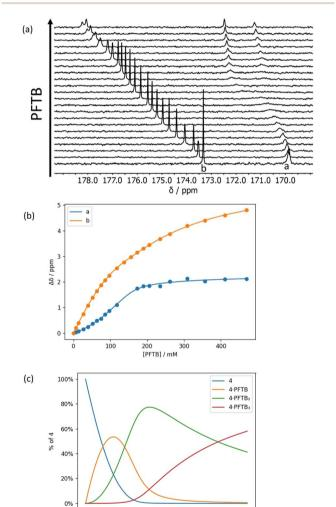
Fig. 10 (a) Partial 176 MHz  $^{13}$ C NMR spectra for titration of perfluorotert-butanol into 4 (90 mM) in n-octane at 298 K. (b) Best fit of the NMR data to a 1:3 binding isotherm ( $K_1$  and  $K_2 > 10^3$  M $^{-1}$  and  $K_3 = 5$  M $^{-1}$ ). (c) Speciation as a function of PFTB concentration.<sup>34</sup>
