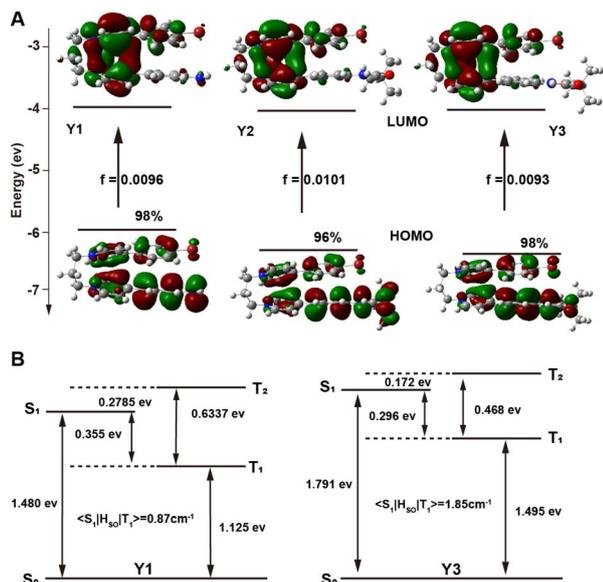
Fig. 5 Quantum chemical calculation of  $Y_n$ . (A) Transition configurations (%), energy level diagrams, and frontier molecular orbital of the  $S_0$ – $S_1$  transition of  $Y_n$  ( $n = 1$ –3). (B) SOC coefficients and energy-level diagrams in  $Y_1$  and  $Y_3$ .
