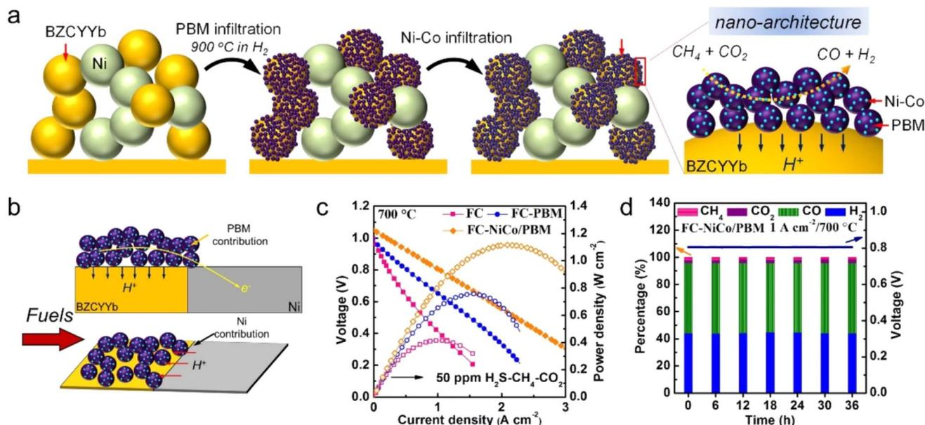
Fig. 17 (a) Schematic preparation procedures of NiCo/PBM catalyst selectively loading on BZCYYb in the porous nickel cermet anode, (b) the role of PBM nanocatalyst and Ni in cermet, (c) electrochemical performance of PCFCs fed with 50 ppm H<sub>2</sub>S-CH<sub>4</sub>/CO<sub>2</sub> fuel using different fuel electrodes and (d) the exhaust gas compositions of FC-NiCo/PBM during continuous 36 h testing.<sup>306</sup> Reproduced with permission.
