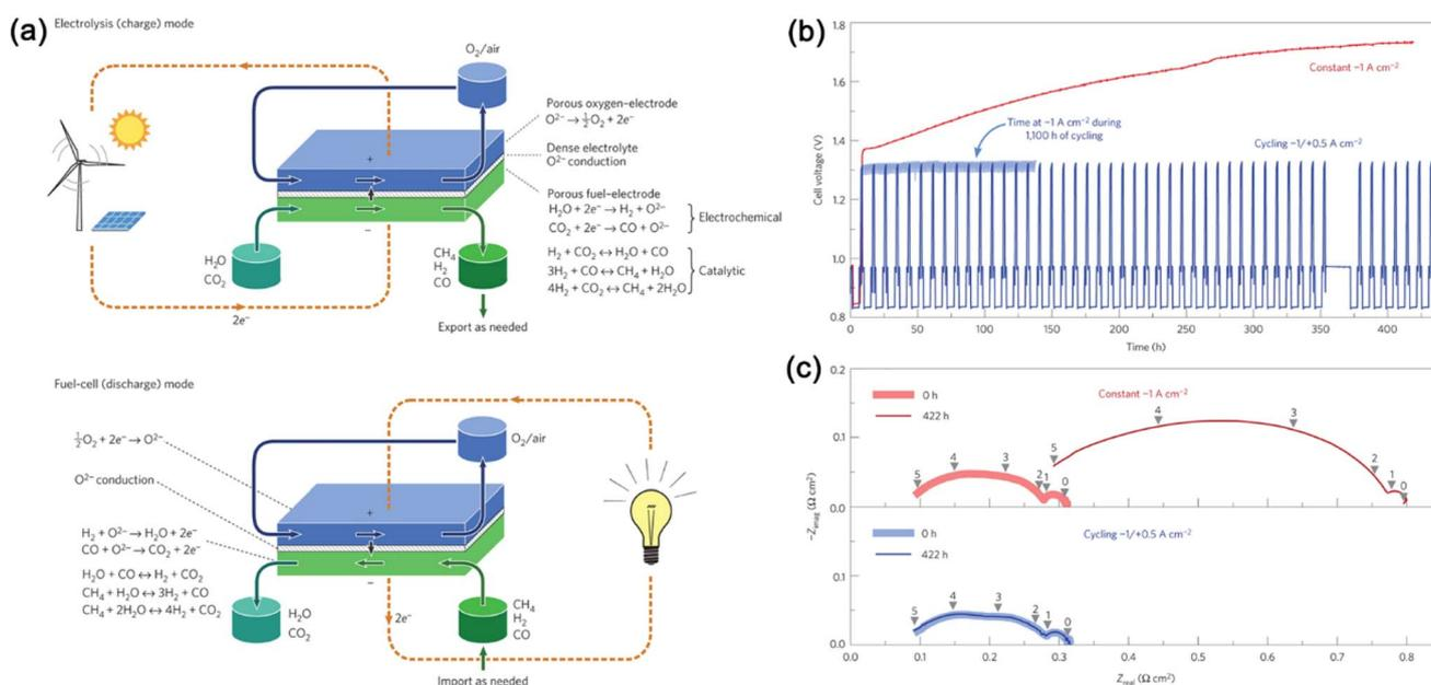
Fig. 14 (a) Schematic illustration of an RSOC, comparison of (b) voltage and (c) impedance spectra responses of an SOC during a constant-current electrolysis test, and a reversible cycling test.<sup>71</sup> Reproduced with permission.
