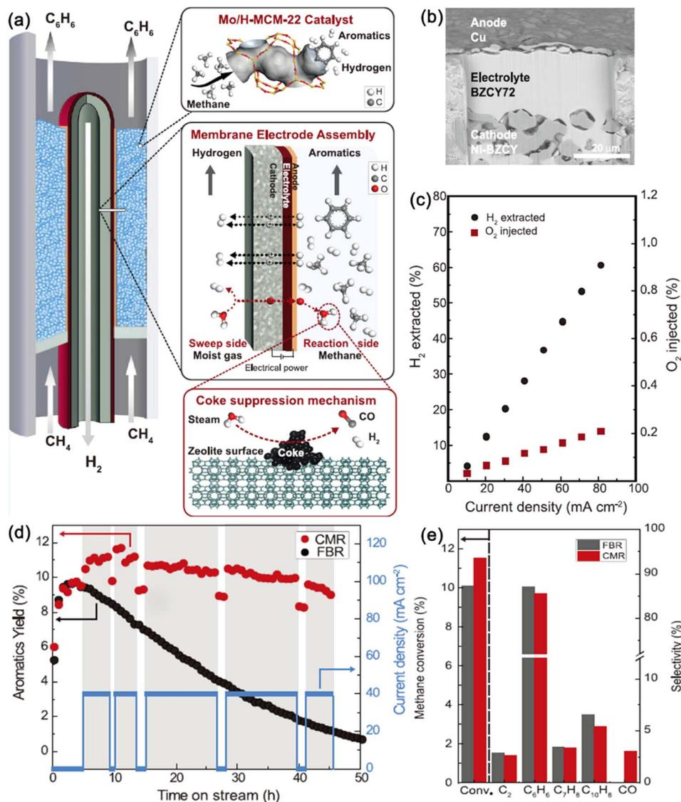
Fig. 16 Co-ionic conductive SEMRs for CH<sub>4</sub> to aromatics conversion: (a) tubular cell configuration and material system, (b) SEM image of MEA based on BZCY electrolyte, (c) percentage of H<sub>2</sub> extracted and O<sub>2</sub> injected versus current density at 700 °C, (d) aromatic yields vs. time and (e) CH<sub>4</sub> conversion.<sup>47</sup> Reproduced with permission.
