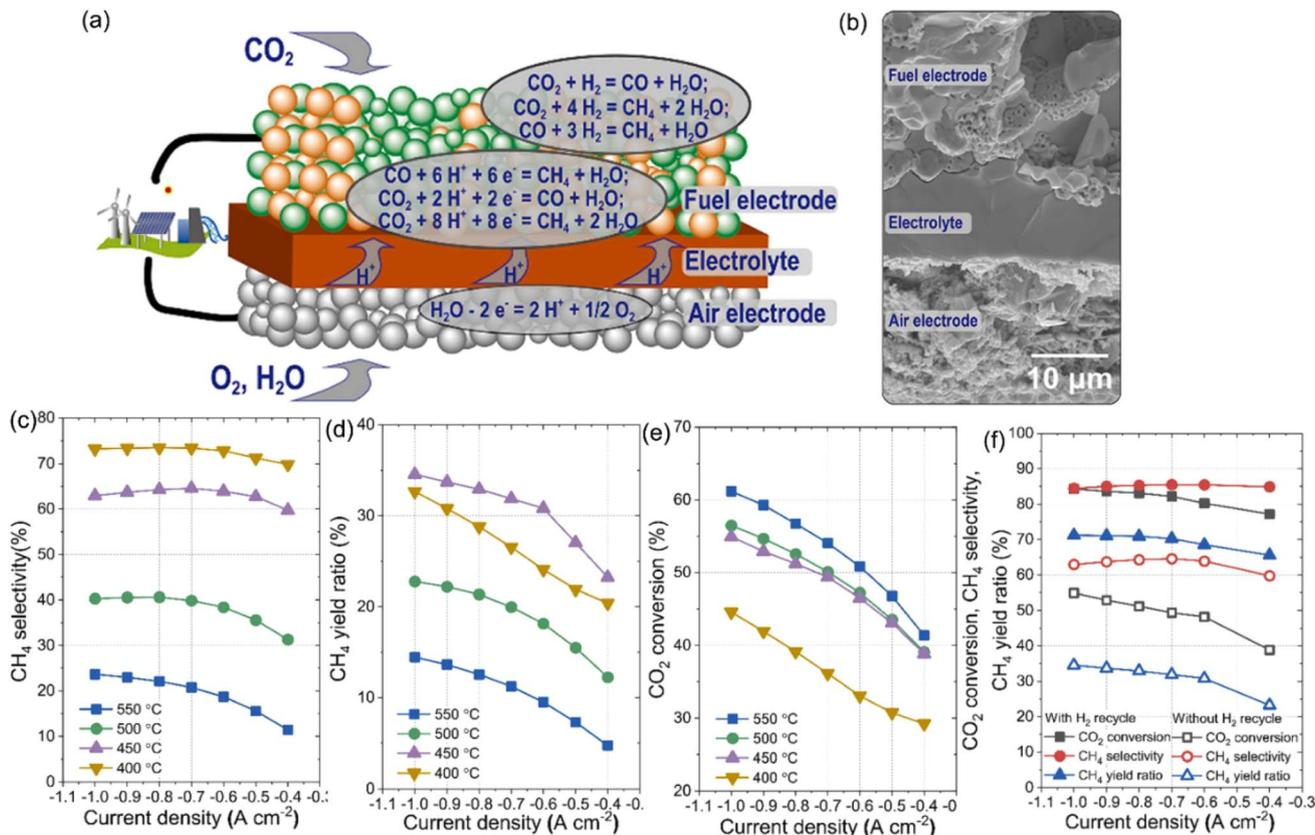
Fig. 19 (a) Schematic illustration of the possible electrochemical and chemical reactions during electrolysis and upgrading  $\text{CO}_2\text{-H}_2\text{O}$  into  $\text{CH}_4$  in the PCEC (b), (c–e) one pass  $\text{CO}_2$  conversion,  $\text{CH}_4$  selectivity, and  $\text{CH}_4$  yields at 400–550 °C, and (f) with  $\text{H}_2$  recycling at 450 °C.<sup>117</sup> Reproduced with permission.
