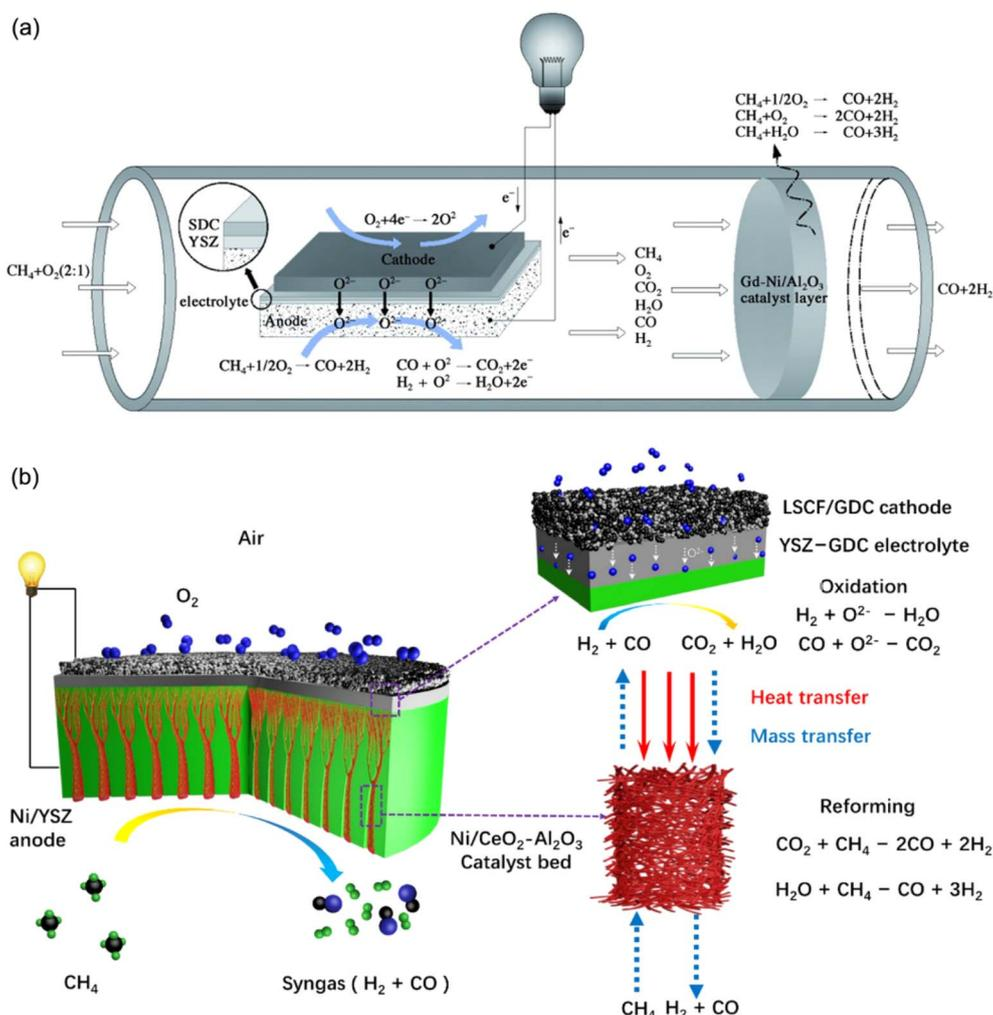
Fig. 11 Different strategies for  $\text{CH}_4$ -fed SEMRs for power and syngas cogeneration: (a) single chamber-SEMR integration with a downstream catalytic partial reformer<sup>50</sup> and (b) thermal and catalytic coupling within the SEMR anode.<sup>198</sup> Reproduced with permission from ref. 50 and <sup>198</sup>.
