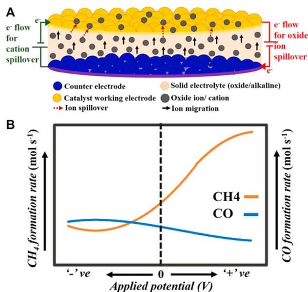
Fig. 26 (A) Schematic of the basic principle of EPOC when ions (oxide ions or cations) are moved to the catalyst of the working electrode<sup>408</sup> and (B) CH<sub>4</sub> and CO production rates when CO<sub>2</sub> hydrogenation is carried out over a range of negative and positive polarization.<sup>390</sup> Reproduced with permission from ref. 390 and 408.
