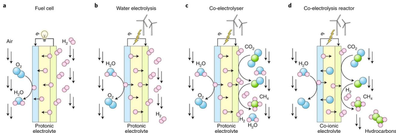
Fig. 15 The different working principles of H-SEMRs: (a) fuel cell, (b) electrolyzer cell, (c) CO<sub>2</sub>/H<sub>2</sub>O co-electrolysis, and (d) co-electrolysis reactor based on co-ionic conductor.<sup>66,265</sup> Reproduced with permission.
