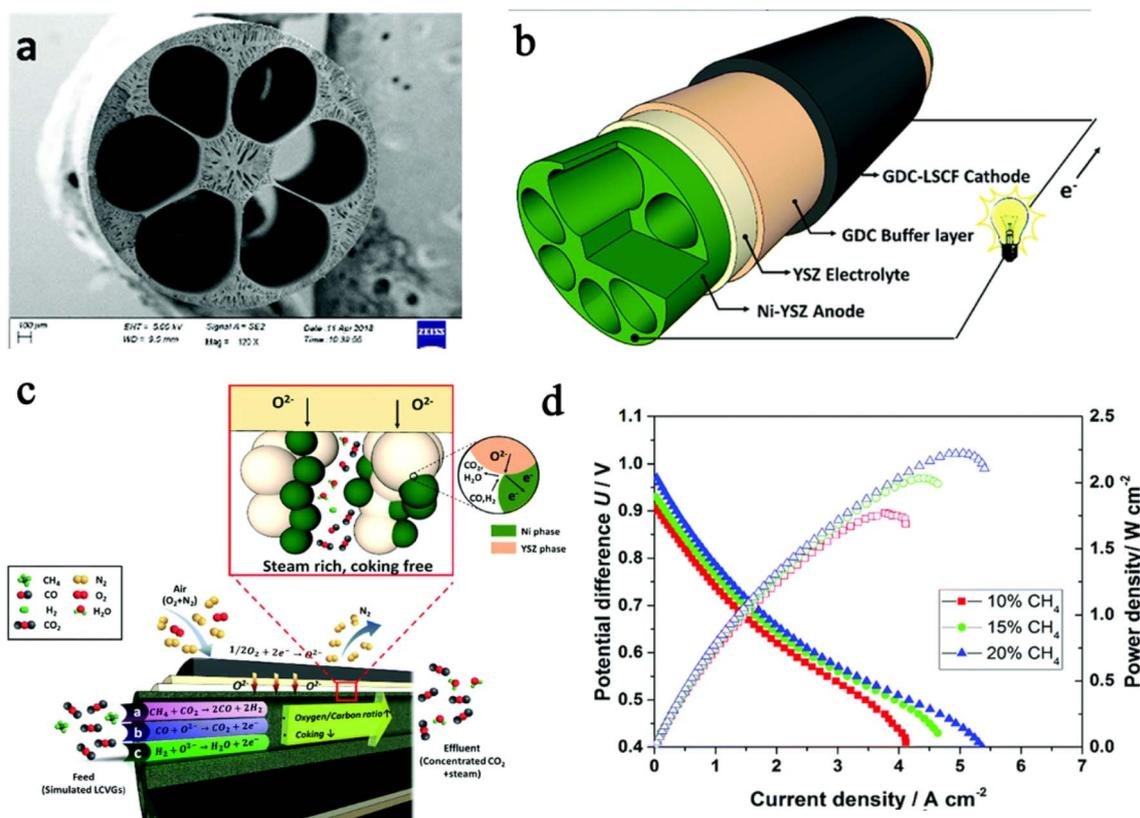
Fig. 22 Novel SEMR (SOFC) design: (a) the micro-monolithic anode support incorporating 6 sub-channels with droplet shapes, (b) full structure simulation, (c) utilizing LCVGs with reactions at triple-phase boundaries, and (d) power density/voltage-current density characteristics with various LCVGs fed as fuels. With permission (open access) from ref. 364.
