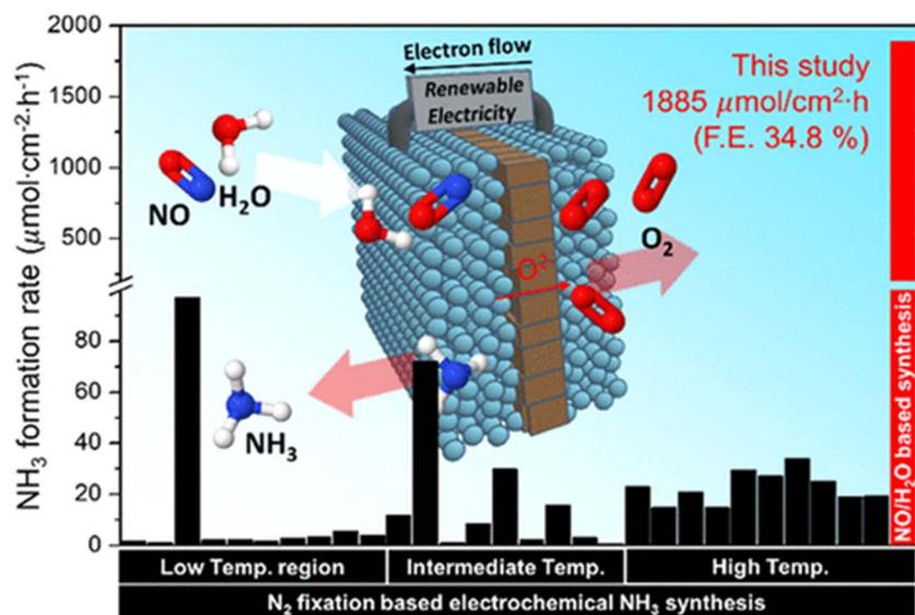
Fig. 8 Schematic illustration of the electrochemical synthesis of  $\text{NH}_3$  from  $\text{NO}$  and  $\text{H}_2\text{O}$  using oxygen-conducting SEMRs and the comparison of  $\text{NH}_3$  yield with other studies operated at low to higher temperatures.<sup>160</sup> Reproduced with permission.
