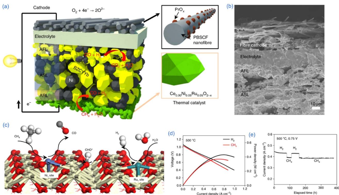
Fig. 10 (a) Schematics of a Ce<sub>0.90</sub>Ni<sub>0.05</sub>Ru<sub>0.05</sub>O<sub>2</sub> catalytic layer modified classic BZCYYb SOFC, (b) cross-sectional SEM image, (c) the synergistic effect of Ni and Ru element for CH<sub>4</sub> and CO<sub>2</sub> activation using DFT calculations, (d) fuel cell performance, and (e) durability.<sup>180</sup> Reproduced with permission.
