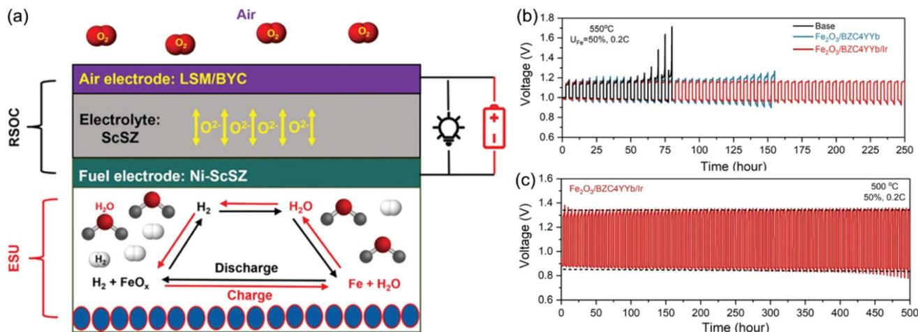
Fig. 13 (a) Cell structure, working principle and cycling performance with different anode fuel materials at  $U_{\text{Fe}} = 50\%$  and  $0.2\text{C}$  ( $10 \text{ mA cm}^{-2}$ ) at  $550 \text{ }^\circ\text{C}$  (b) and  $500 \text{ }^\circ\text{C}$  (c) of a solid oxide iron–air battery.<sup>251</sup> Reproduced with permission (open access).
