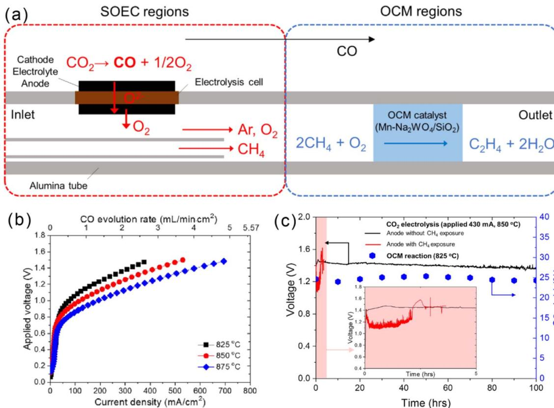
Fig. 7 (a) Schematic diagram of integrating the  $\text{CO}_2$  electrolysis with the OCM process in a successive two-stage reactor design, (b) SOEC performance and (c) durability comparison.<sup>154</sup> Reproduced with permission.
