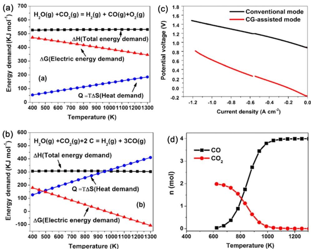
Fig. 4 Thermodynamic calculation of the required energy for CO<sub>2</sub>–H<sub>2</sub>O co-electrolysis without (a) and with (b) carbon fuel in the anode, (c) comparison of the  $I$ – $V$  curves of the electrolysis cell, and (d) temperature-dependence of anode outlet gas composition.<sup>138</sup> Reproduced with permission.
