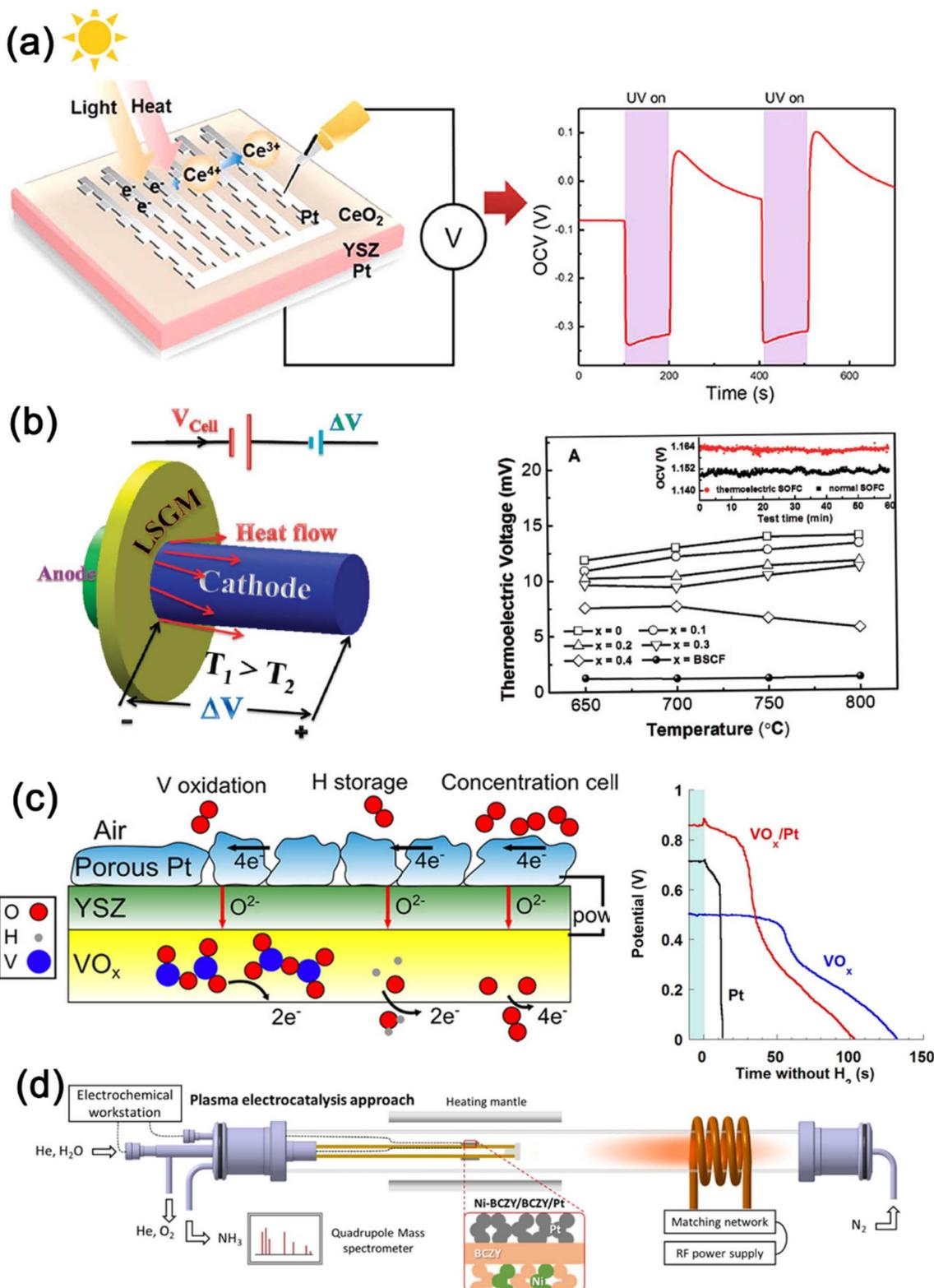
Fig. 23 Process-intensified SEMRs using different external energy sources: (a) light-induced cell voltage increase in solid oxide photo-electrochemical cells,<sup>373</sup> (b) thermoelectric SOFCs,<sup>377</sup> (c) SEMRs intensified by H<sub>2</sub> energy storage in the anode<sup>51</sup> and (d) plasma intensified SEMRs for N<sub>2</sub> activation and NH<sub>3</sub> synthesis.<sup>378</sup> Reproduced with permission from individual reference-related publishers.
