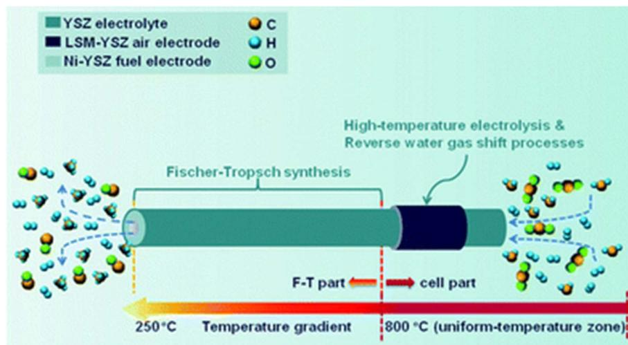
Fig. 3 The proposed cell structure design for coupling the low temperature F–T process and high temperature co-electrolysis process.<sup>124</sup> Reproduced with permission.
