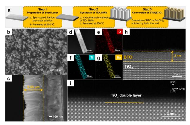
Fig. 1 Characterization of the BTO@TiO<sub>2</sub> photoanode. (a) Schematic of the synthesis of BTO@TiO<sub>2</sub>. (b) SEM images of BTO@TiO<sub>2</sub> with the top (c) and side view, (d-g) EDX elemental distribution of a single BTO@TiO<sub>2</sub> NW, (h) the HAADF-STEM image of BTO@TiO<sub>2</sub>, and (i) an annealed surface layer of BTO.
