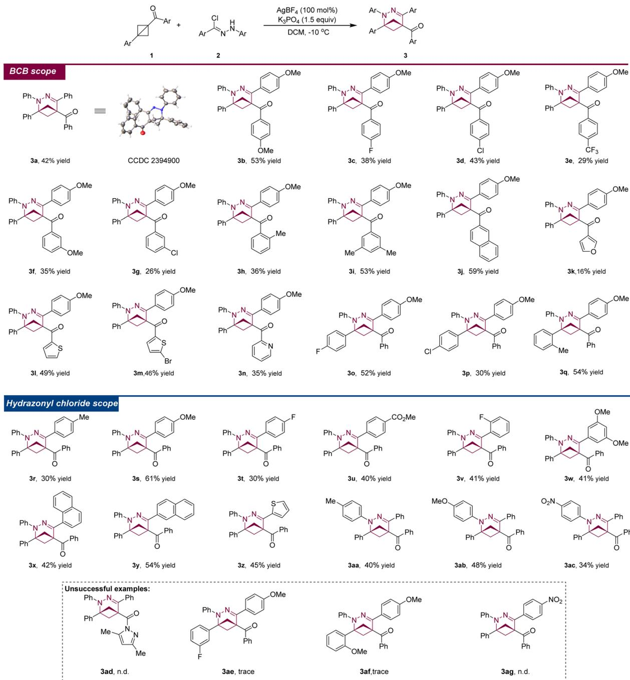
Scheme 2 Exploration of substrate scope. Reaction conditions: **1** (0.3 mmol), **2** (0.1 mmol),  $K_3PO_4$  (0.15 mmol),  $AgBF_4$  (0.1 mmol, 100 mol%), 3 Å molecular sieves (50 mg), DCM (1 mL),  $-10\text{ }^\circ\text{C}$ , Ar, 1 h. For details, see the ESI†.
