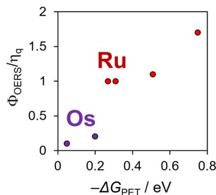
Fig. 1  $\Phi_{OERS}/\eta_q$  values of Ru(II) and Os(II) tris-diimine complexes using BIH as a reductant, as a function of the driving force for photoinduced electron-transfer: produced using the data reported in ref. 6.
