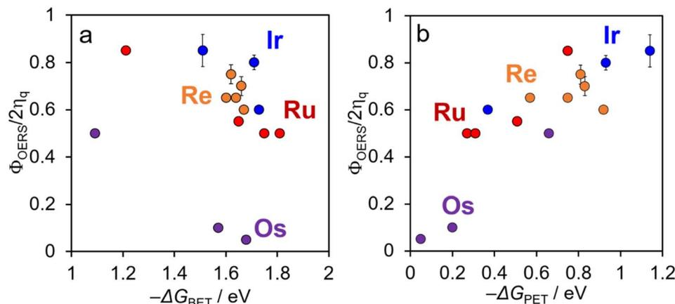
Fig. 8 Plots of  $\Phi_{\text{OERS}}/2\eta_{\text{q}}$  for  $[\text{Re}(\text{PR}_3)_2]^+$  (orange),  $[\text{Ir}(\text{C}^{\wedge}\text{N})_2(\text{N}^{\wedge}\text{N})]^+$  (blue), and Ru(II) (red), and Os(II) (purple) tris(diimine) complexes as a function of the driving force for (a) back-electron-transfer between OERSs and  $\text{BIH}^{*+}$  ( $-\Delta G_{\text{BET}}$ ) and (b) photoinduced electron-transfer ( $-\Delta G_{\text{PET}}$ ).
