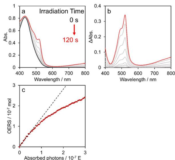
Fig. 6 (a) Time-dependent visible absorption changes of an Ar-saturated DMA solution containing  $[\text{Re}(\text{PEt}_3)_2]^+$  (0.2 mM) and BIH (0.1 M) during irradiation with light at  $\lambda_{\text{ex}} = 436 \text{ nm}$  ( $5.2 \times 10^{-9} \text{ E s}^{-1}$ ) and (b) calculated difference absorption spectra before and after irradiation. (c) Relationship between the number of absorbed photons and the concentration of OERSs from  $[\text{Re}(\text{PEt}_3)_2]^+$  in solution.
