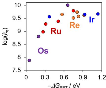
Fig. 7 Relationship between  $-\Delta G_{\text{PET}}$  and  $k_q$  for  $[\text{Re}(\text{PR}_3)_2]^+$  (orange),  $[\text{Ir}(\text{C}^{\wedge}\text{N})_2(\text{N}^{\wedge}\text{N})]^+$  (blue), and reported Ru(II) (red) and Os(II) (purple) tris- $(\text{X}_2\text{bpy})$  ( $\text{X}_2\text{bpy} = 4,4' - \text{X}_2 - \text{bpy}$ ) complexes and  $[\text{Os}(\text{CF}_3\text{bpy})_3]^{2+}$ .
