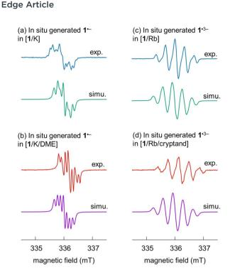
Fig. 6 Experimental and simulated EPR spectra of (a and b) the monoanion  $\mathbf{1}^{-}$  and (c and d) trianion  $\mathbf{1}^{\cdot 3-}$  in solution under different conditions. Experimental spectra were re-scaled individually to yield comparable intensities.
