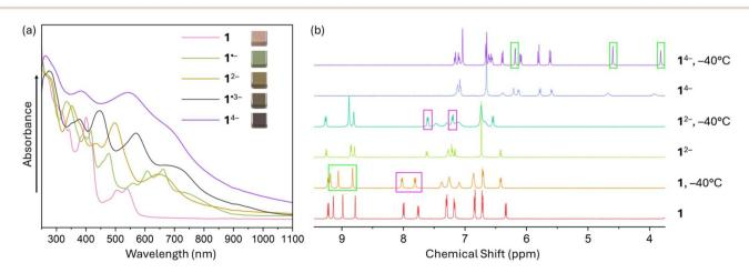
Fig. 2 (a) UV-vis-NIR absorption spectra of TPP and its *in situ* generated anions by Rb metal in THF at 25 °C. (b)  $^{1}$ H NMR spectra of TPP and its *in situ* generated dianion and tetraanion by Rb metal in THF- $d_8$  at 25 °C and -40 °C.
