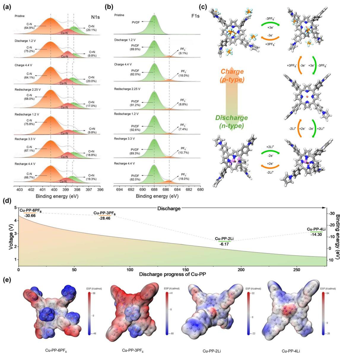
Fig. 6 (a) N 1s and (b) F 1s of *ex situ* XPS spectra for PPCMP-Cu at different charge states. (c) The structure evolution of the repeating unit of PPCMP-Cu during the charge/discharge process. (d) The discharge pathway was obtained from simulations. (e) The optimized different active sites were obtained via the MESP method.
