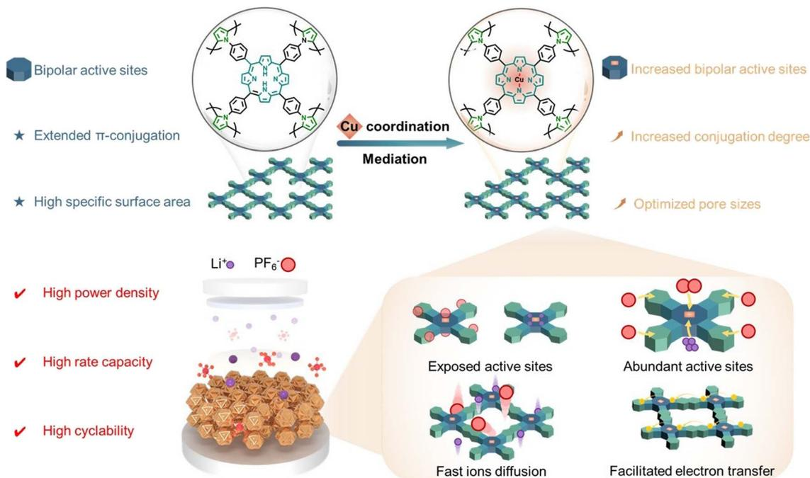
Fig. 1 Schematic illustration of the advantages of the Cu-mediated bipolar-type CMP with abundant exposed active sites, high conjugation degree, and optimized pore sizes for high-performance LIB cathode materials.
