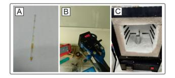
Fig. 3 (A) Photo of a capillary with p-xylene after heating to 500 °C for 5 min. (B) Photo of an experiment with induction heating. (C) Muffle furnace with maximum heating temperature of 1200 °C. Chamber volume: 3.6 liters.
