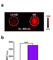
Fig. 2 (a) PA tissue-mimicking phantom images of LG-AB and the turn-over product AB (5  $\mu$ M) in 1:1 v/v MeCN/PBS (pH = 7.4). (b) Quantified data from panel (a). n=3. Error bars = SD. Statistical analysis was performed using a two-tailed t-test ( $\alpha=0.05$ , \*\*P < 0.01, \*\*\*P < 0.001).
