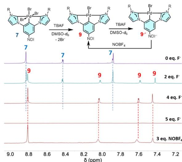
Fig. 3 Selected region of the  $^1\text{H}$  NMR spectra of complex 7 in  $\text{DMSO-}d_6$  upon the addition of increasing amounts of  $\text{TBAF} \cdot 3\text{H}_2\text{O}$  showing the formation of the Pd(II) complex 9, and finally the paramagnetic species  $9^{\cdot-}$ . Subsequent addition of  $\text{NOBF}_4$  reoxidizes  $9^{\cdot-}$  to 9 (bottom spectrum).
