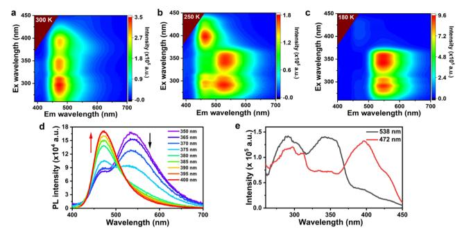
Fig. 2 Excitation-fluorescence mapping of 2 in CH<sub>3</sub>OH at (a) 300 K, (b) 250 K, and (c) 180 K, with a concentration of 33.3  $\mu$ M. (d) PL spectra of 2 in CH<sub>3</sub>OH at 250 K with an  $\lambda_{ex}$  range of 350–400 nm. (e) Excitation spectra of 2 in CH<sub>3</sub>OH at 250 K, emission wavelength: 472 nm (red) and 538 nm (black)
