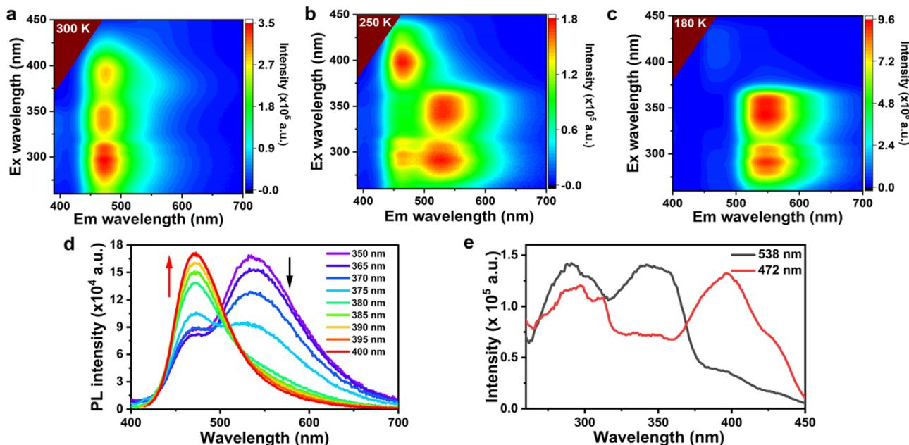
Fig. 2 Excitation-fluorescence mapping of **2** in  $\text{CH}_3\text{OH}$  at (a) 300 K, (b) 250 K, and (c) 180 K, with a concentration of 33.3  $\mu\text{M}$ . (d) PL spectra of **2** in  $\text{CH}_3\text{OH}$  at 250 K with an  $\lambda_{\text{ex}}$  range of 350–400 nm. (e) Excitation spectra of **2** in  $\text{CH}_3\text{OH}$  at 250 K, emission wavelength: 472 nm (red) and 538 nm (black).
