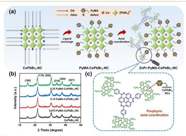
Fig. 1 (a) Schematic diagram for the preparation process of the pristine, PyMA-modified, and ZnPr-PyMA-modified CsPbBr $_3$  perovskite NCs and their corresponding detailed structures (including the interaction of porphyrin, PyMA ligand, and perovskite NC). (b) XRD patterns of the pristine and modified CsPbBr $_3$  NCs with different PyMA contents. (c) The magnified schematic diagram of the molecular structure of ZnPr and its axial interaction with the PyMA ligand.
