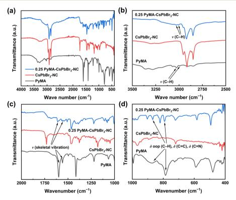
Fig. 5 (a) FT-IR spectra of PyMA, CsPbBr $_3$ -NC, and 0.25 PyMA-CsPbBr $_3$ -NC. The zoomed-in FT-IR spectra in the (b) 2500–3500 cm $^{-1}$ , (c) 1000–2000 cm $^{-1}$ , and (d) 400–1000 cm $^{-1}$  regions.
