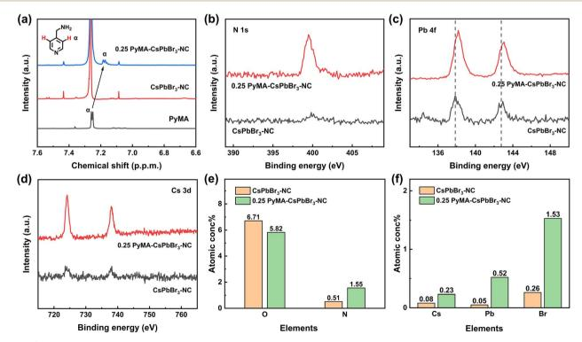
Fig. 6 (a) <sup>1</sup>H NMR spectra of PyMA, CsPbBr<sub>3</sub>-NC, and 0.25 PyMA-CsPbBr<sub>3</sub>-NC (in CDCl<sub>3</sub>). XPS spectra of (b) N 1s, (c) Pb 4f, and (d) Cs 3d of the pristine CsPbBr<sub>3</sub>-NC and 0.25 PyMA-CsPbBr<sub>3</sub>-NC and their schematic diagrams of the content changes of (e) O and N and (f) Cs, Pb, and Br elements.
