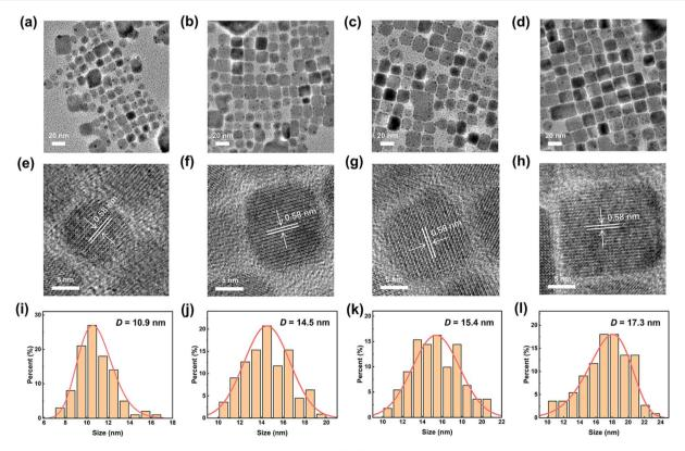
Fig. 2 (a)–(d) TEM images, (e)–(h) high-resolution TEM images, and (i)–(l) corresponding particle size distribution diagrams for the pristine  $CsPbBr_3$ -NC and 0.075, 0.15, and 0.25  $PyMA-CsPbBr_3$ -NCs. D is the average particle size.
