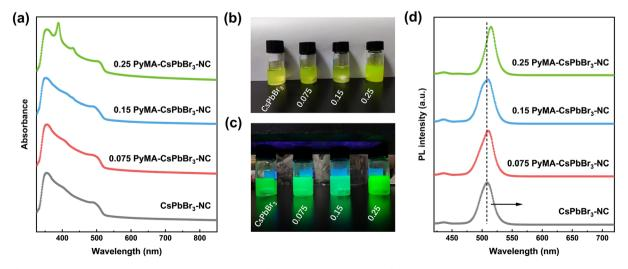
Fig. 3 (a) UV-vis spectra, images under (b) natural light and (c) 365 nm UV lamp, and (d) emission spectra for CsPbBr<sub>3</sub> NCs without and with different contents of PyMA treatment.
