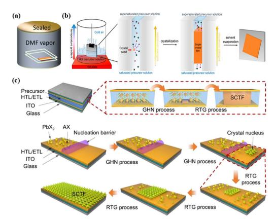
Fig. 1 (a) Schematic diagram of saturated solvent vapor assisted method.<sup>42</sup> (b) Bottom-up saturation techniques to induce crystallization.<sup>38</sup> (c) Schematic of the nucleation and growth process of the FAPbBr<sub>3</sub> SCTFs by room temperature gradient crystallization method.<sup>46</sup>
