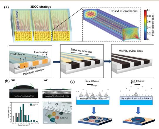
Fig. 2 (a) Schematics of fluid flow and illustration of the growth process of perovskite crystals within the closed 3D microchannel.<sup>47</sup> (b) Contact angle measurements and reproducibility counts of single crystals size on PTAA-coated ITO glass and MeO-2PACz-coated ITO glass.<sup>55</sup> (c) Growth mechanism of MAPbl<sub>3</sub> films on TiO<sub>2</sub>/FTO and PTAA/ITO substrates.<sup>58</sup>
