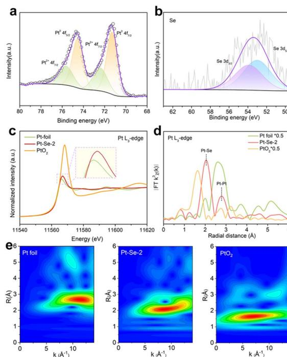
Fig. 2 XPS spectra of (a) Pt 4f and (b) Se 3d for Pt–Se-2. (c) Pt L<sub>3</sub>-edge XANES spectra and (d) corresponding FT-EXAFS spectra for Pt–Se-2 in reference to Pt foil and PtO<sub>2</sub>. (e) WT for the *k*<sup>3</sup>-weighted EXAFS of the Pt L<sub>3</sub>-edge for Pt–Se-2, Pt foil, and PtO<sub>2</sub>.
