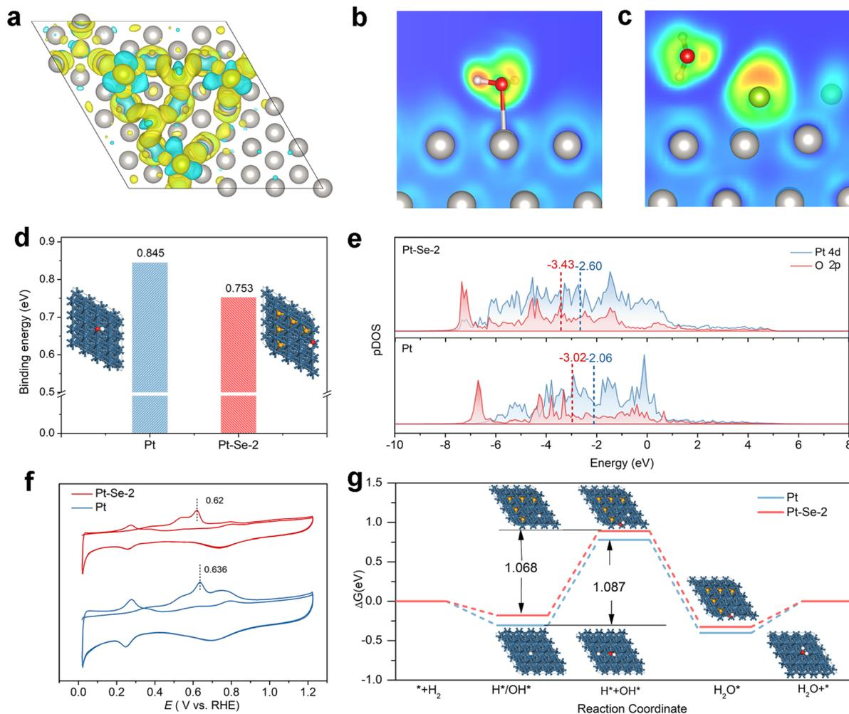
Fig. 5 (a) Calculated differential charge density for Pt–Se-2. ELF evaluation for H<sub>2</sub>O adsorption on (b) Pt and (c) Pt–Se-2. (d) The adsorption energy of OH\* on Pt and Pt–Se-2 with the corresponding optimal theoretical structure. (e) The p-DOS of Pt 4d orbitals and O 2p orbitals in Pt and Pt–Se-2. (f) CO stripping curves of Pt and Pt–Se-2 in CO-saturated 0.1 M KOH. (g) The reaction path of Pt and Pt–Se-2, and the corresponding optimized structure.
