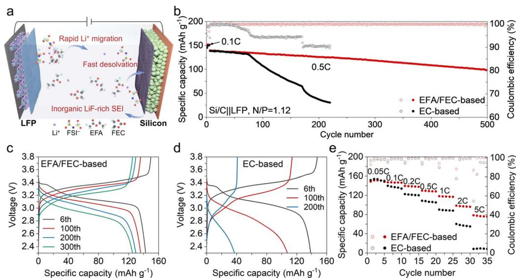
Fig. 5 Electrochemical performance of Si/C||LFP cells at room temperature. (a) Schematic illustration of interfacial Li<sup>+</sup> transport kinetics and interfacial stability of the Si/C||LFP battery. (b) Cycling performance at 0.5C after five activation cycles at 0.05C (1C = 170 mA g<sup>-1</sup>). Corresponding charge/discharge curves of Si/C||LFP cells using (c) EFA/FEC-based and (d) EC-based electrolytes. (e) Rate performance using EFA/FEC-based and EC-based electrolytes.
