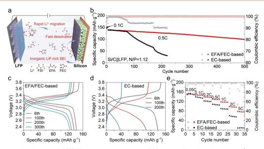
Fig. 5 Electrochemical performance of Si/C||LFP cells at room temperature. (a) Schematic illustration of interfacial Li<sup>+</sup> transport kinetics and interfacial stability of the Si/C||LFP battery. (b) Cycling performance at 0.5C after five activation cycles at 0.05C ( $1C = 170 \text{ mA g}^{-1}$ ). Corresponding charge/discharge curves of Si/C||LFP cells using (c) EFA/FEC-based and (d) EC-based electrolytes. (e) Rate performance using EFA/FEC-based and EC-based electrolytes.
