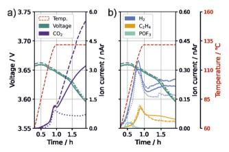
Fig. 4 Changes during thermal abuse for three cells (solid, dashed, dotted) with 0.1 vol% VC in electrolyte and a formation rate of 1C. (a) Temperature, open circuit voltage and  $CO_2$  (m/z 44, purple). (b) Temperature (red), open circuit voltage (green) and gases with  $H_2$  (m/z 2, blue),  $C_2H_4$  (m/z 26, yellow) and  $POF_3$  (m/z 104, cyan). Signals have been normalized to m/z 36 (normalized to argon, nAr).
