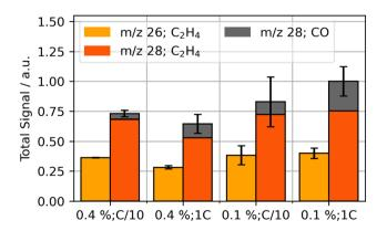
Fig. 1 Integrated signal of detected gases CO (m/z 28, grey) and C<sub>2</sub>H<sub>4</sub> (m/z 26, yellow; m/z 28, orange) from the start of the formation process to 12 hours for various VC concentrations (vol%) and formation currents
