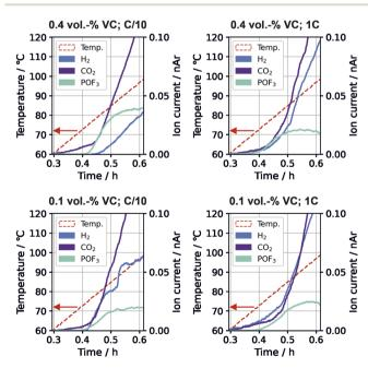
Fig. 3 Temperature and gas evolution of  $H_2$  (m/z 2, blue),  $CO_2$  (m/z44, purple), and POF3 (m/z 104, cyan) for cells with different VC content and formation rate during the thermal stress test. Signals have been normalized to m/z 36 (normalized to argon, nAr).
