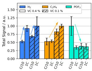
Fig. 2 Selected integrated gas signals during the heat-up phase without holding time during the thermal stress test up to 132 °C at SOC 50 for various VC concentrations (vol%) and formation currents:  $H_2$  (m/z 2, blue),  $C_2H_4$  (m/z 26, yellow) and POF $_3$  (m/z 104, cyan), average signal intensity for every investigated analyte normalized to 1.
