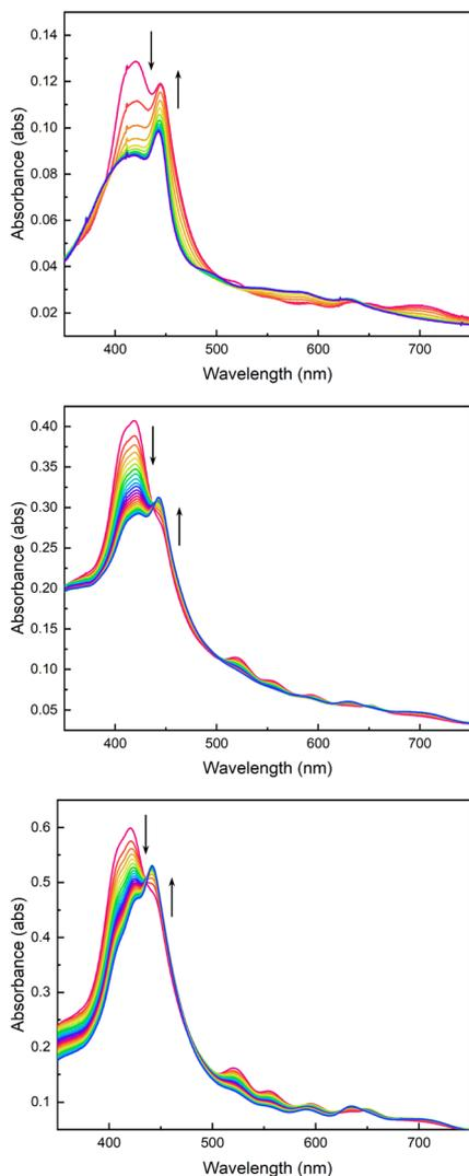
Fig. 8 Time-dependent UV-vis spectra collected every 10 minutes during the metalation of 10 (top), 20 (middle), and 30 (bottom) deposition cycle [Zr<sub>m</sub>BDC][H<sub>2</sub>(tcpp)] films with Mn(HMDS)<sub>2</sub>.
