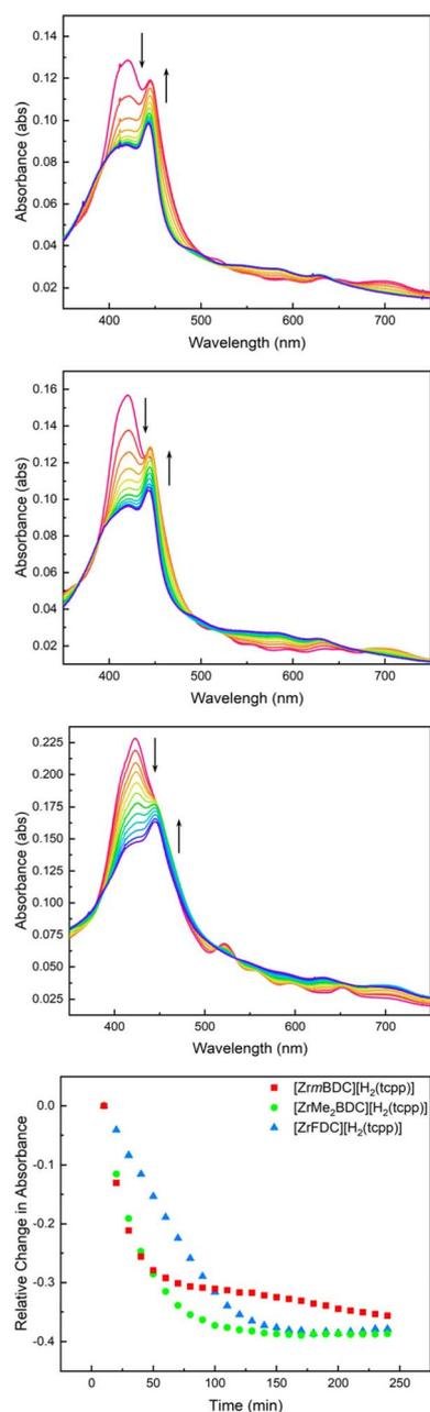
Fig. 7 Time-dependent UV-vis spectra collected every 10 minutes during the metalation of 10 deposition cycle  $[\text{Zr}m\text{BDC}][\text{H}_2(\text{tcpp})]$  (top),  $[\text{ZrMe}_2\text{BDC}][\text{H}_2(\text{tcpp})]$  (middle), and  $[\text{ZrFDC}][\text{H}_2(\text{tcpp})]$  (bottom) films with  $\text{Mn}(\text{HMDS})_2$ . The change in freebase Soret absorbance as a function of time illustrates a marked cage dependence of metalation.
