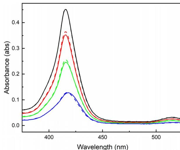
Fig. 2 UV-vis absorption spectra of a  $[ZrmBDC][H_2(tcpp)]$  thin film grown to 5 (blue), 10 (green), 15 (red), and 20 (black) deposition cycles. After every 5 cycles the film was exposed to the solution containing the target anion 10 additional times and a UV-vis spectra was collected (dashed line = additional 10 exposures).
