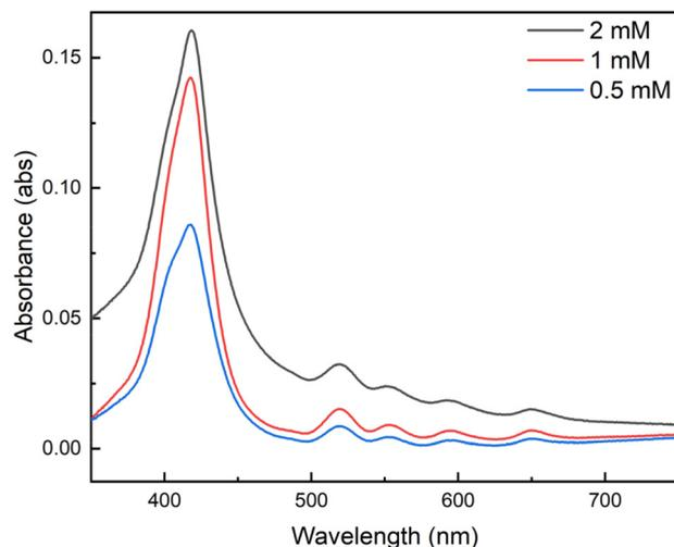
Fig. 4 UV-vis spectra of optically transparent porous thin films grown to 5 deposition cycles using 0.5 mM solutions (blue), 1.0 mM solutions (red), and 2.0 mM solutions (black) of  $[\text{Zr}(\text{mBDC})][\text{OTf}]_4$  and  $[\text{HNEt}_3]_4[\text{H}_2(\text{tcpp})]$  in methanol.
