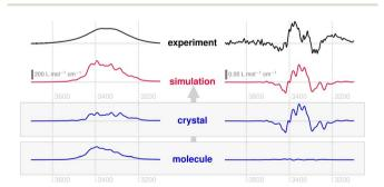
Fig. 5 Solid-state IR absorption spectra (left) and VCD spectrum (right) of compound 2, obtained from KBr pellets (black) as well as predicted from periodic AIMD-NVPT calculations (red). The experimental spectra have been scaled to approximately match the intensities. The lower shaded panel shows the calculated subspectra that make up the simulated spectrum corresponding to molecular and crystal chirality (blue).
