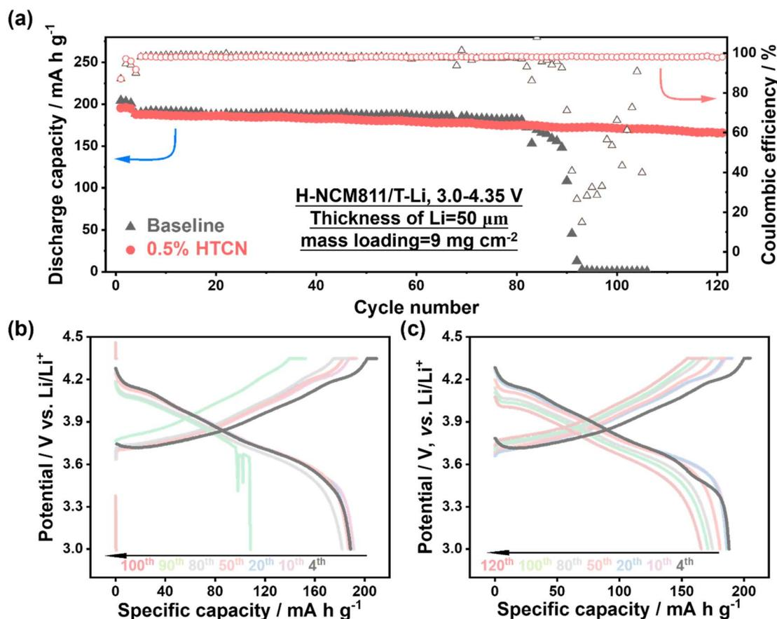
Fig. 6 (a) Cycling stability of H-NCM811/Li full cells in various electrolytes at 0.2C for the initial three cycles and 1C for the subsequent cycles. Selected charge/discharge curves cycled in (b) baseline and (c) HTCNC-containing electrolytes.
