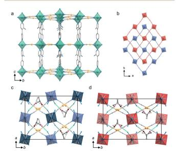
Fig. 2 The perspective view (a) and double interpenetration (b) of the Fe·<sup>i</sup>PrOH framework. The lattice conformation of Fe·<sup>i</sup>PrOH at 100 K (c) and 298 K (d) viewed along the *c*-axis. The two-fold disordered <sup>i</sup>PrOH molecules are marked in distinct shades of color and the green dashed lines stand for the host–guest H-bonding interactions. The black boxes indicate the unit cell dimensions. Hydrogen atoms are omitted for clarity.
