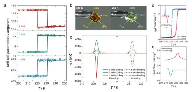
Fig. 4 (a) Crystallographic axis parameters (circle) for Fe<sup>-i</sup>PrOH in the temperature range of 200–250 K. Solid lines indicate the best-fitting results using the sigmoidal function. (b) The crystal images of Fe. PrOH recorded at 210 and 250 K. (c) The calculated thermal expansion coefficients according to unit cell parameters. (d) Variable-temperature molar magnetic susceptibility measured in the settle mode for  $Fe^{-i}$ PrOH. (e) The DSC curves of Fe-iPrOH at 10 K min<sup>-1</sup>.
