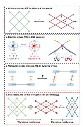
Fig. 1 Schematics of ATE regimes. (a) ATE *via* the vibrational mechanism in a wine-rack framework; (b) ATE *via* the electronic mechanism in an SCO complex; (c) ATE *via* collective motion in a dynamic molecular crystal; (d) three-in-one strategy for switchable ATE in this work.
