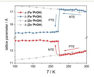
Fig. 3 Temperature-dependent unit cell vectors (a-axis and b-axis) in  ${\bf Fe}\cdot^{\bf i}{\bf PrOH}$  and its Zn-analogue.
