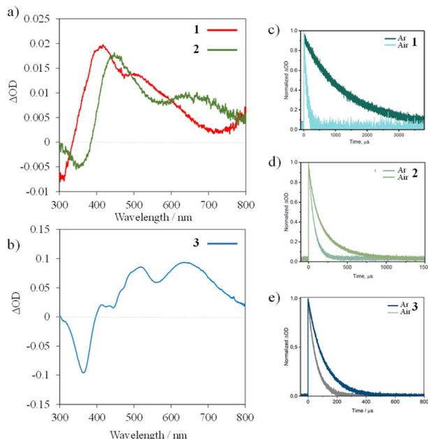
Fig. 5 (a) and (b) Transient absorption spectra of compounds **1**, **2** and **3** upon excitation at 355 nm (30 mJ per pulses, *ca.* 10 ns duration) for **1** and **2**, and at 450 nm (13 mJ per pulse) for **3** with nanosecond pulses in deaerated acetonitrile solution at room temperature, time-integrated over 1  $\mu\text{s}$ . (c) 410 nm, (d) 450 nm and (e) 520 nm decays of the normalized ESA bands for the three compounds.
