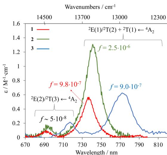
Fig. 3 Spin-flip absorption spectra of 1, 2 and 3 complexes in acetonitrile ( $c = 7.7 \text{ mM}$ ). Band assignment according to (CASSCF(7,12)/FIC-NEVPT2) calculations (see text and Fig. S23†). The oscillator strength ( $f$ ) has been calculated according to eqn (2).
