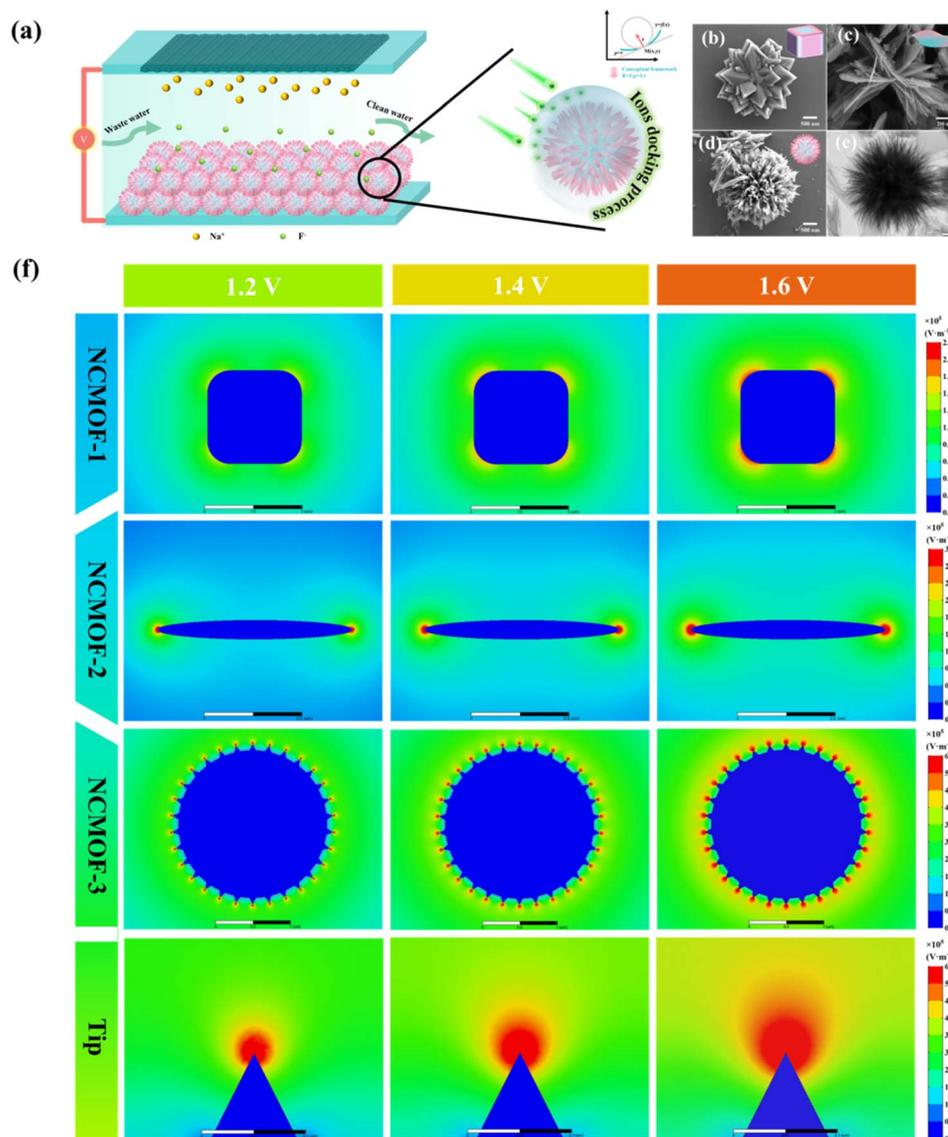
Fig. 1 (a) Diagram of the CDI process using urchin-like NCMOF-3 with 3D interconnection network structure as the anode.  $K$ ,  $\rho$  and  $r$  denote the curvature, curvature radius and framework radius, respectively. SEM of (b) NCMOF-1, (c) NCMOF-2, and (d) NCMOF-3. (e) TEM of NCMOF-3. (f) Results of simulation for electric field distribution in NCMOF-1 ( $\rho = 1450$  nm), NCMOF-2 ( $\rho = 500$  nm), NCMOF-3 and the tip of the NCMOF-3 ( $\rho = 50$  nm).
