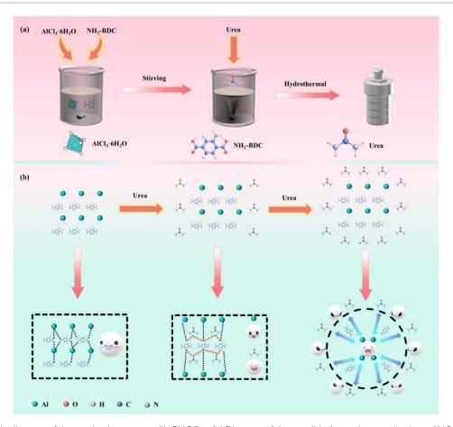
Fig. 2 (a) Schematic diagram of the synthesis process of NCMOF-2, (b) Diagram of the possible formation mechanism of NCMOF-1, NCMOF-2, NCMOF-3.
