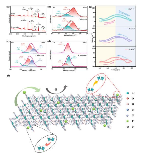
Fig. 5 (a) XPS survey spectrum, (b) N 1s, and (c) O 1s of NCMOF-3 before and after adsorption. (d) High-resolution F 1s XPS spectra of NCMOF-3 after adsorption. (e)  $\triangle m$  of NCMOF-3 electrode from EQCM-D during CV at different scan rates. (f) Diagram of the adsorption mechanism of  $F^-$ .
