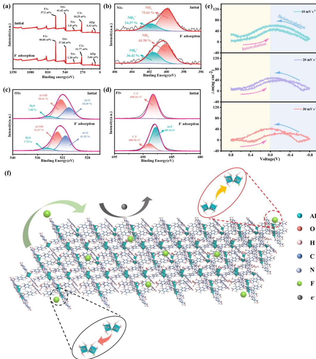
Fig. 5 (a) XPS survey spectrum, (b) N 1s, and (c) O 1s of NCMOF-3 before and after adsorption. (d) High-resolution F 1s XPS spectra of NCMOF-3 after adsorption. (e)  $\Delta m$  of NCMOF-3 electrode from EQCM-D during CV at different scan rates. (f) Diagram of the adsorption mechanism of  $F^-$ .
