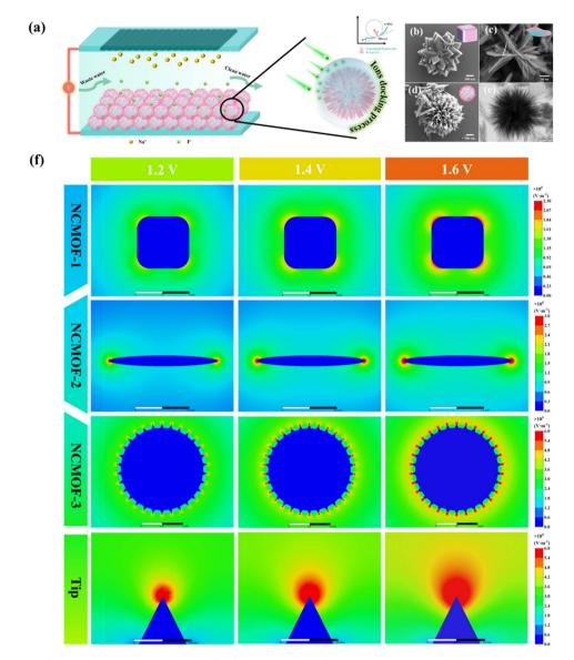
Fig. 1 (a) Diagram of the CDI process using urchin-like NCMOF-3 with 3D interconnection network structure as the anode. K,  $\rho$  and r denote the curvature, curvature radius and framework radius, respectively. SEM of (b) NCMOF-1, (c) NCMOF-2, and (d) NCMOF-3. (e) TEM of NCMOF-3. (f) Results of simulation for electric field distribution in NCMOF-1 ( $\rho = 1450 \text{ nm}$ ), NCMOF-2 ( $\rho = 500 \text{ nm}$ ), NCMOF-3 and the tip of the NCMOF-3 ( $\rho = 1450 \text{ nm}$ ). = 50 nm).
