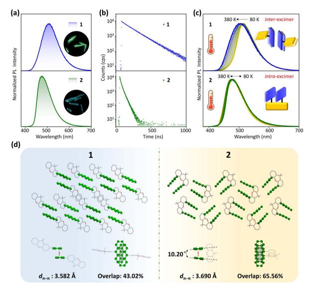
Fig. 2 (a) PL spectra and (b) time-resolved PL spectra of crystals 1 and 2. (c) Temperature-dependent PL spectra of crystals 1 and 2. (d) Molecular packing structures of crystals 1 and 2
