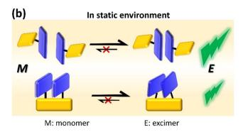
Fig. 4 (a) PLQYs,  $k_r$ s and  $k_{nr}$ s of crystals 1 and 2. (b) Schematic diagram of inter-excimer and intra-excimer in a static environment. In a static environment, due to the restriction of the intramolecular template, intra-excimer could only assume a metastable state, while inter-excimer could readily relax to the most stable equilibrium geometry.
