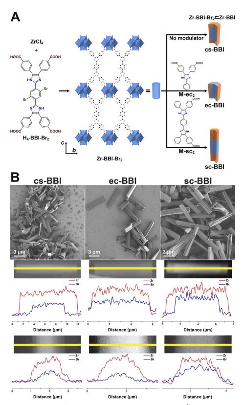
Fig. 4 Illustration of binary domain Zr-BBI MOF syntheses and crystal structure of Zr-BBI-Br<sub>2</sub> ( $Zr^{4+}$ , blue polyhedra; C, black spheres; O, red spheres; Br, green spheres; H omitted for clarity) (A); SEM images for binary Zr-BBI MOFs (B, top); SEM-EDS line-scans along longitudinal (B, middle) and transverse (B, bottom) directions.
