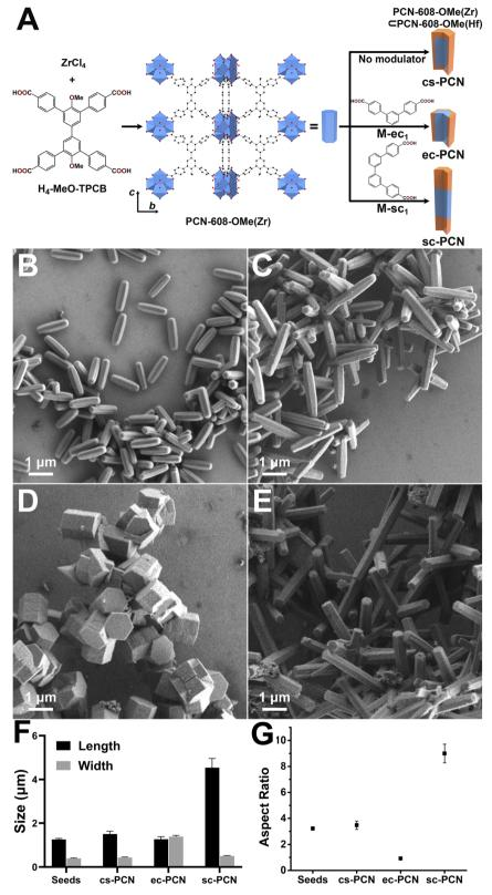
Fig. 2 Illustration of binary domain PCN MOF syntheses and crystal structure of PCN-608-OMe(Zr) ( $Zr^{4+}$ , blue polyhedra; C, black spheres; O, red spheres; H omitted for clarity) (A); SEM images for PCN-608-OMe seeds (B), cs-PCN (C), ec-PCN (D), SC-PCN (E); sizes (F) and aspect ratios (G) of seeds and binary domain PCN MOFs (each point in (F) and (G) is the average of 100 counts and the error bars represent the standard deviation of the mean).
