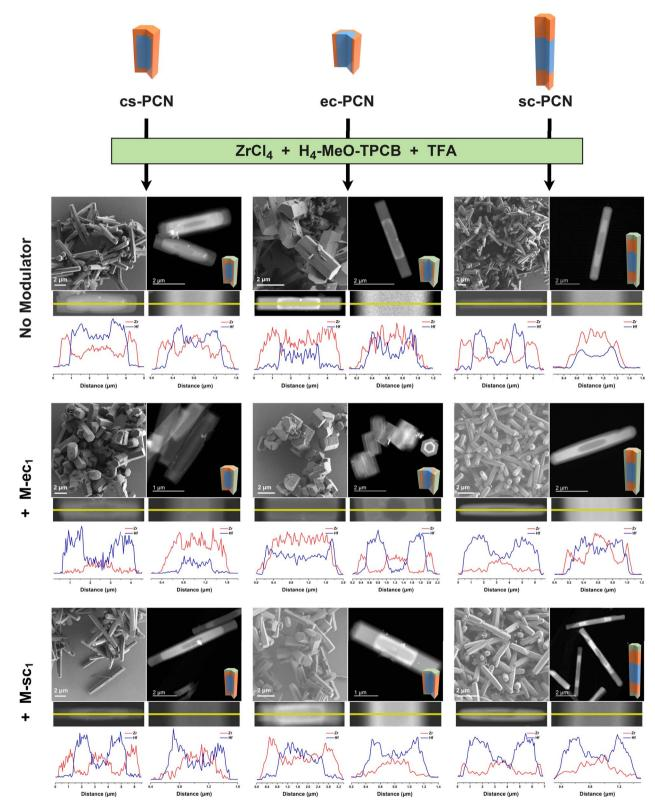
Fig. 5 SEM, HAADF images and longitudinal (left) and transverse (right) STEM-EDS line-scans for nine ternary domain PCN MOFs synthesized with different modulators using binary cs-PCN, ec-PCN and sc-PCN as seeds.
