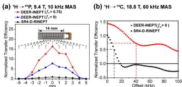
Fig. 2 Comparisons of experimental transfer efficiencies of DEER-INEPT, SR4-D-RINEPT and PRESTO. (a)  $^1\text{H} \rightarrow ^{31}\text{P}$  transfer in ADP with the sample packed at different rotor positions; (b)  $^1\text{H} \rightarrow ^{13}\text{C}$  transfer in  $^{13}\text{C}_\alpha$ -glycine with varying  $^1\text{H}$  resonance offset. The methods, MAS frequencies and magnetic fields are denoted in each figure. The details of NMR experiments are provided in the ESI.†
