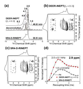
Fig. 4 Experiments on dehydrated HY zeolites. (a) 1D  $^{1}$ H $^{27}$ Al} spectra and deconvolution of the  $^{1}$ H signals. The proton-detected 2D  $^{1}$ H $^{-27}$ Al correlation spectra from (b) DEER-INEPT ( $f_{\rm w}=0.5$ ) and (c) SR4-D-RINEPT. (d)  $^{1}$ H $^{-27}$ Al distance measurements by fitting the signal buildup curves at  $\delta_{\rm iso}(^{1}$ H) = 3.6 ppm. The experiments are operated at 18.8 T and 20 kHz MAS, with details provided in the ESI.†
