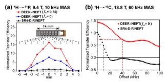
Fig. 2 Comparisons of experimental transfer efficiencies of DEER-INEPT, SR4-D-RINEPT and PRESTO. (a)  $^1\text{H} \rightarrow ^{31}\text{P}$  transfer in ADP with the sample packed at different rotor positions; (b)  $^1\text{H} \rightarrow ^{13}\text{C}$  transfer in  $^{13}\text{C}_{\alpha}$ -glycine with varying  $^1\text{H}$  resonance offset. The methods, MAS frequencies and magnetic fields are denoted in each figure. The details of NMR experiments are provided in the ESI.†
