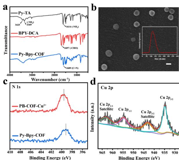
**Fig. 1** (a) FTIR spectra of Py-TA (gray), BPy-DCA (red) and the Py-Bpy-COF (blue). (b) SEM image of the Py-Bpy-COF. Scale bar = 100 nm. The inset photograph was the corresponding DLS size distribution histogram. (c and d) XPS spectra of (c) N 1s and (d) Cu 2p of PB-COF-Cu<sup>2+</sup>.
