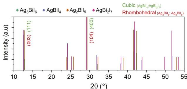
Fig. 4 XRD patterns extracted from crystallographic libraries for SBI compounds.  $\text{Ag}_3\text{BiI}_6$  (CCDC 1776740)<sup>62</sup> (blue),  $\text{AgBiI}_4$  (CCDC 1671019)<sup>62</sup> (violet),  $\text{Ag}_2\text{BiI}_5$  (JCPDS card # 00-035-1025) (orange) and  $\text{AgBi}_2\text{I}_7$  (PDF card # 00-034-1372) (pink).
