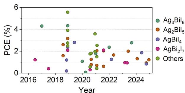
Fig. 2 Efficiency of Ag<sub>3</sub>BiI<sub>6</sub>, Ag<sub>2</sub>BiI<sub>5</sub>, AgBiI<sub>4</sub>, AgBi<sub>2</sub>I<sub>7</sub>, and other SBI-related compounds reported over the years (full table is given in ESI, Table S1†).
