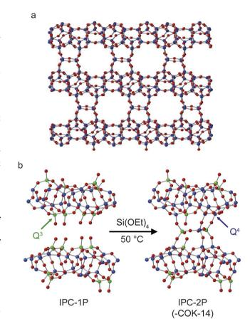
Fig. 1 Schematics showing (a) the structure of IPC-2/COK-14 and (b) the process of forming IPC-2P through rection of TEOS with the layered silicate IPC-1P. Red atoms are oxygen, green are  $Q^3$  silicon and blue are  $Q^4$  silicon. An expanded view of one layer of the structure of IPC-1P is given in Fig. S3.1 of the ESI.†
