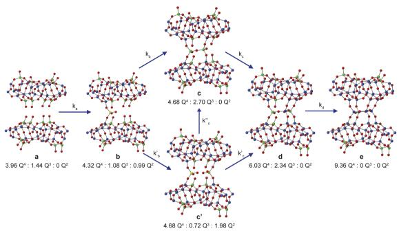
Fig. 5 Schematic showing the proposed mechanism of intercalation of Si(OH)<sub>4</sub> into the layers of IPC-1P. The ratios of NMR-active <sup>29</sup>Si Q<sup>4</sup>, Q<sup>3</sup> and Q<sup>2</sup> species for each of the structural models **a**, **b**, **c**, **c**', **d** and **e** are given. Oxygen atoms are shown in red, and Q<sup>2</sup>, Q<sup>3</sup> and Q<sup>4</sup> Si atoms in yellow, green and blue, respectively.
