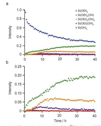
Fig. 3 (a) Plot showing the intensities of the <sup>29</sup>Si liquid-state NMR signals for TEOS and all monomeric hydrolysis products formed in the reaction with IPC-1P as a function of time. (b) Expanded view of the data in (a), highlighting the very low concentration of Si(OH)<sub>4</sub>. The data are normalised such that the total intensity of the monomeric species at t = 0 is equal to 1 (i.e., the low levels of oligomeric species present are neglected).
