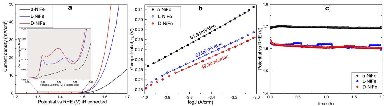
Fig. 2 (a) Linear sweep voltammetry data for the a-NiFe ( $0.40 \text{ mg cm}^{-2}$ ), D-NiFe ( $0.25 \text{ mg cm}^{-2}$ ) and L-NiFe ( $0.5 \text{ mg cm}^{-2}$ ) samples on Ni foil; in the inset a detailed image of the redox waves for the different oxides is provided. (b) Tafel plot for the different chiral oxides (a-NiFe, D-NiFe and L-NiFe samples). (c) Stability test for 2 hours at  $10 \text{ mA cm}^{-2}$ .
