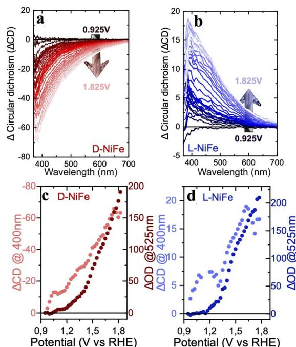
Fig. 4 Spectroelectrochemical analysis of chiral oxides (L-NiFe and D-NiFe) at an applied potential in the 0.9–1.8 V *vs.* RHE range. (a and b) Chiral activity extracted from the CD signal for both oxides. (c and d) CD difference correlated with the applied potential during the OER in a KOH (1 M) electrolyte.
