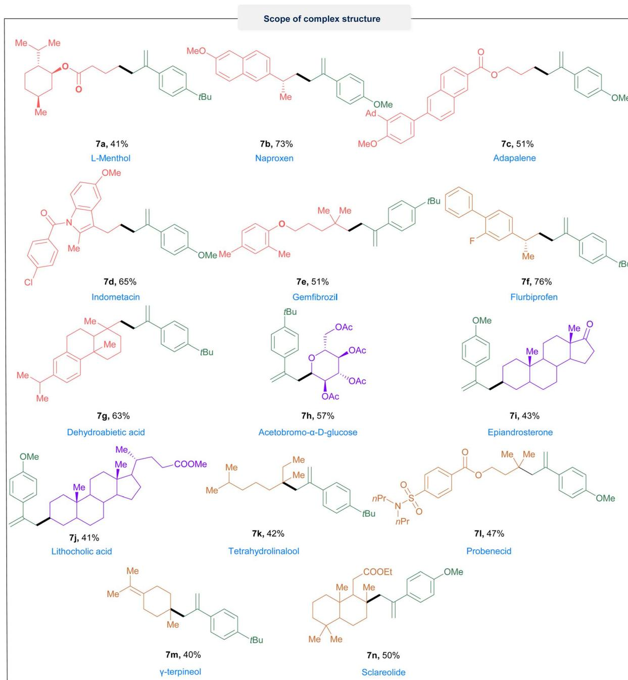
Fig. 3 Modification of structurally complex molecules. Reactions were performed with 0.2 mmol of **1**, 0.4 mmol of **2**, 0.2 M of TBAB, and 4 mL of DMA in an undivided cell at R. T. and constant current  $i = 4$  mA,  $5.2$  F mol<sup>-1</sup>.
