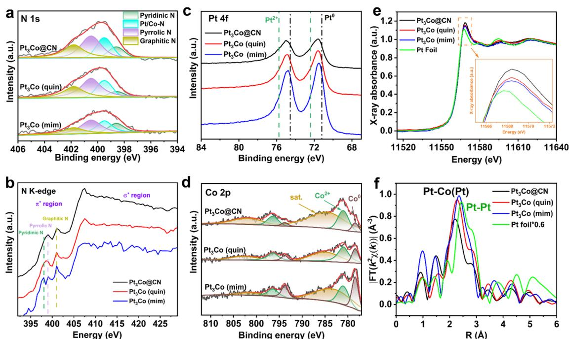
Fig. 3 Characterization of Pt<sub>3</sub>Co (N sources). (a) N 1s XPS, (b) N K-edge NEXAFS, (c) Pt 4f XPS and (d) Co 2p XPS spectra of Pt<sub>3</sub>Co@CN, Pt<sub>3</sub>Co (quin), Pt<sub>3</sub>Co (mim). (e) Pt L<sub>3</sub>-edge XANES and (f) FT-EXAFS spectra of Pt<sub>3</sub>Co@CN, Pt<sub>3</sub>Co (quin), and Pt<sub>3</sub>Co (mim) with Pt foil as reference.
