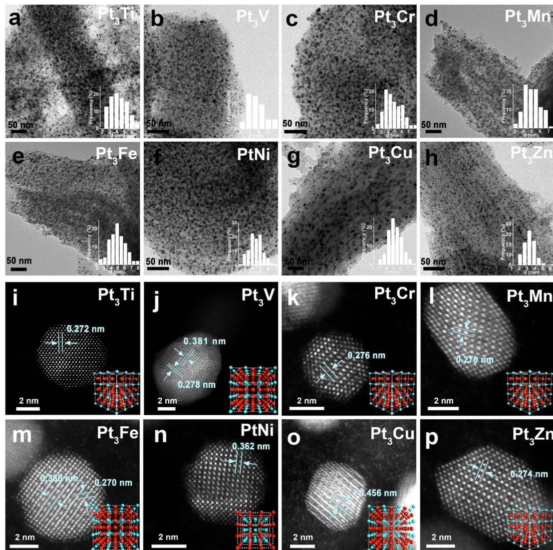
Fig. 4 Characterization of Pt-M IMCs. (a–h) TEM images and (i–p) AC-HAADF-STEM images of Pt<sub>3</sub>Ti, Pt<sub>3</sub>V, Pt<sub>3</sub>Cr, Pt<sub>3</sub>Mn, Pt<sub>3</sub>Fe, PtNi, Pt<sub>3</sub>Cu and Pt<sub>3</sub>Zn, respectively. Insets in (a–h) show the corresponding statistical particle size distributions. Insets in (i–p) show the atomic model corresponding to the crystal face.
