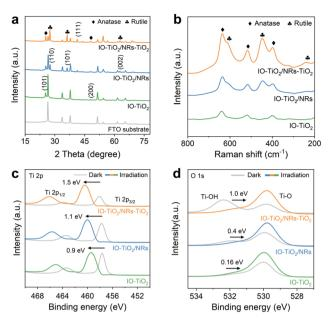
Fig. 3 (a) XRD patterns of FTO,  $IO-TiO_2$ ,  $IO-TiO_2/NRs$ , and  $IO-TiO_2/NRs-TiO_2$ , (b) Raman spectra of  $IO-TiO_2$ ,  $IO-TiO_2/NRs$  and  $IO-TiO_2/NRs-TiO_2$ . XPS spectra of  $IO-TiO_2$ ,  $IO-TiO_2/NRs$  and  $IO-TiO_2/NRs-TiO_2$  in dark and irradiated states: (c) Ti 2p and (d) O 1s.
