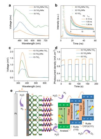
Fig. 5 (a) PL spectra, (b) TRPL spectra, (c) SPV spectra, and (d) photocurrent response of IO-TiO2, IO-TiO2/NRs and IO-TiO2/NRs-TiO<sub>2</sub>. (e) Schematic diagram of the band alignment and charge transfer in an IO-TiO<sub>2</sub>/NRs-TiO<sub>2</sub> heterojunction, and the light scattering and electron transport in the IO-TiO2/NRs-TiO2 photoanode for water splitting
