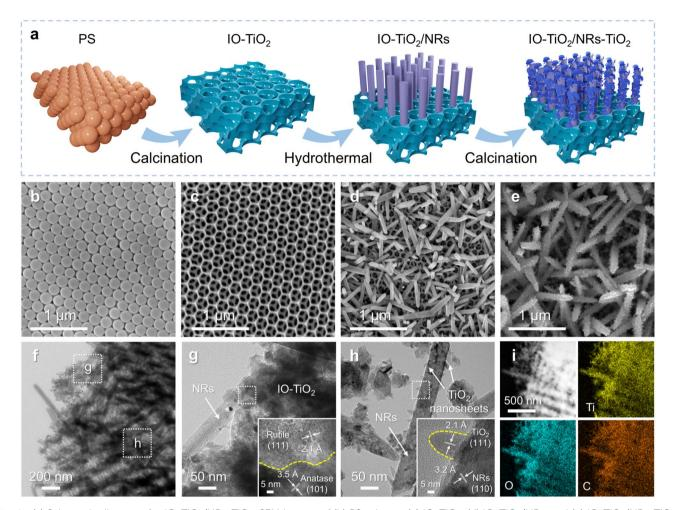
Fig. 2 (a) Schematic diagrams for IO-TiO<sub>2</sub>/NRs-TiO<sub>2</sub>. SEM images of (b) PS spheres, (c) IO-TiO<sub>2</sub>, (d) IO-TiO<sub>2</sub>/NRs, and (e) IO-TiO<sub>2</sub>/NRs-TiO<sub>2</sub>. TEM images of (f) IO-TiO<sub>2</sub>/NRs-TiO<sub>2</sub>, (g) the anatase/rutile heterojunction, and (h) the rutile crystal surface heterojunction. (i) EDS element mapping of IO-TiO<sub>2</sub>/NRs-TiO<sub>2</sub>.
