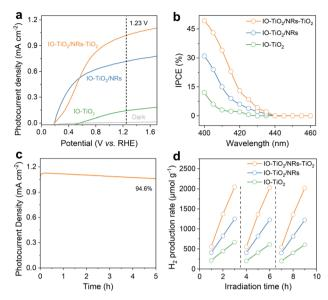
Fig. 4 (a) Linear sweep voltammetry (LSV) curves and (b) incident photon to current conversion efficiency (IPCE) of IO-TiO<sub>2</sub>, IO-TiO<sub>2</sub>/NRs and IO-TiO<sub>2</sub>/NRs-TiO<sub>2</sub>. (c) Long-term photocurrent-time curves of IO-TiO<sub>2</sub>/NRs-TiO<sub>2</sub>. (d) The cycling photocatalytic H<sub>2</sub>-evolution test of IO-TiO<sub>2</sub>, IO-TiO<sub>2</sub>/NRs and IO-TiO<sub>2</sub>/NRs-TiO<sub>2</sub>.
