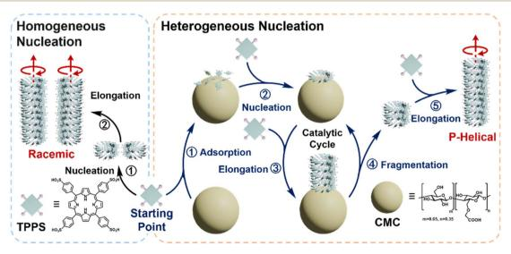
Scheme 1 Schematic representation of the competitive pathways of TPPS homogeneous nucleation and heterogeneous nucleation with CMC as the nucleating agent.
