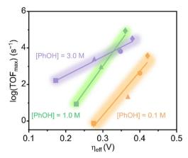
Fig. 8 Scaling relationships for Fe21–Fe23 and Fe1 at different concentrations of phenol.  $\diamondsuit=$  Fe1,  $\bigcirc=$  Fe21,  $\Delta=$  Fe22,  $\square=$  Fe23. The slopes of the lines are purple = 10.3 dec V $^{-1}$ , green = 28.2 dec V $^{-1}$ , and orange = 24.10 dec V $^{-1}$ .
