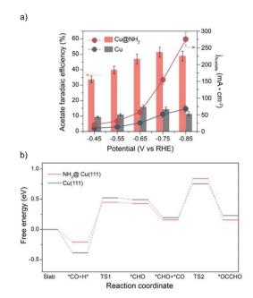
Fig. 4 (a) Acetate FE and partial current density for CO reduction on  $Cu@NH_2$  and Cu recorded in CO-saturated 1.0 M KOH solution. (b) Free energy diagram of the CO reduction mechanism showing \*CO hydrogenation to \*CHO and the subsequent coupling with another \*CO to \*OCCHO on  $Cu@NH_2(111)$  and Cu(111). Adapted with permission from ACS Catal. 2023, 13, 3532–3540. Copyright 2023 American Chemical Society.
