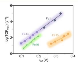
Fig. 7 Scaling relationships for iron hangman porphyrins Fe14–Fe16 and Fe1 showing the effect of phenol (PhOH) concentration. For Fe14–Fe16, [PhOH] = 2, 4, 10, 20, and 40 mM were tested. For Fe1, [PhOH] = 0.1, 0.75, 3.0 M were used. In all cases, a higher phenol concentration led to a higher TOF $_{\rm max}$ . The slopes of the linear regions are 15.58, 11.65, and 18.08 dec V $^{-1}$  for Fe1/Fe14, Fe15, and Fe16, respectively.
