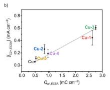
Fig. 3 (a) Electrocatalytic performance of the best-performing NHC-CDI-modified Cu catalyst (Cu<sub>GDE</sub>-3) and a reference Cu catalyst  $(Cu_{GDE})$  in a GDE-based electrolysis setup at -1.1 V vs. RHE, and (b) partial current density for multicarbon products,  $|j_{C_2+,ECSA}|$ , as a function of the accumulated surface charge,  $Q_{\text{an,ECSA}}$  at  $\Delta E = 1.6$  V. Adapted with permission from J. Am. Chem. Soc. 2024, 146, 13034-13045. Copyright 2024 American Chemical Society.
