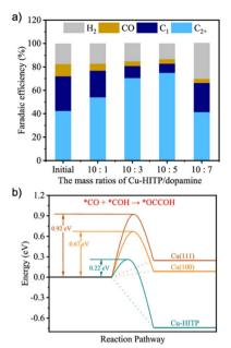
Fig. 6 (a) Comparison of CO<sub>2</sub>RR performances of Cu-HITP with different PDA coating amounts at -1.2 V vs. RHE. (b) Free energy diagram for forming the C-C bond on the Cu-HITP model. Adapted with permission from ACS Catal., 2022, 12, 7986-7993. Copyright 2022 American Chemical Society
