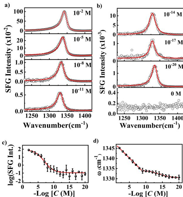
Fig. 2 (a and b) ppp SFG spectra of different concentrations of NTP in the  $\text{NO}_2$  stretching region. (c) The  $\log(\text{SFG Int.})$  and (d)  $\omega$  values of samples self-assembled by a range of concentrations of NTP solutions are plotted against concentration.  $10^{-2}$ ,  $10^{-5}$ ,  $10^{-8}$ ,  $10^{-11}$ ,  $10^{-14}$ ,  $10^{-17}$ ,  $10^{-20}$ , 0 M and the symbol “ $C$ ” represent the concentration of the solution that was used to prepare the SAMs.
