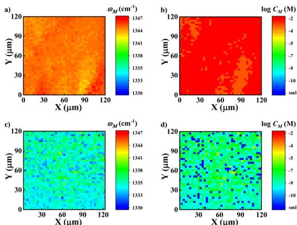
Fig. 5 Images constructed with the  $\nu_{\text{NO}_2}$  frequency (a and c) and its corresponding surface microzone concentration ( $C_M$ ) (b and d). (a) and (b) Sample prepared with  $C = 10^{-2}$  M; (c) and (d) sample prepared with  $C = 10^{-8}$  M. The symbol “C” represents the concentration of the solution that was used to prepare the SAMs. sml: single-molecule level.
