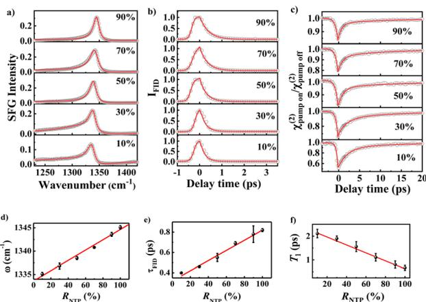
Fig. 4 (a) The ppp SFG spectra in the  $\text{NO}_2$  stretching region. (b) SFG-FID spectra of  $\nu_{\text{NO}_2}$ . (c) The ppp  $\chi^{(2)}$  decay of  $\nu_{\text{NO}_2}$ . (d) The  $\omega$ , (e)  $\tau_{\text{FID}}$ , and (f)  $T_1$  are plotted against  $R_{\text{NTP}}$ .
