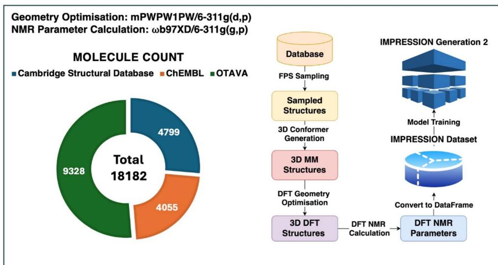
Fig. 1 Workflow for training IMPRESSION-Generation 2 including DFT methodology and training and testing dataset sources. Full details can be found in the ESI.†
