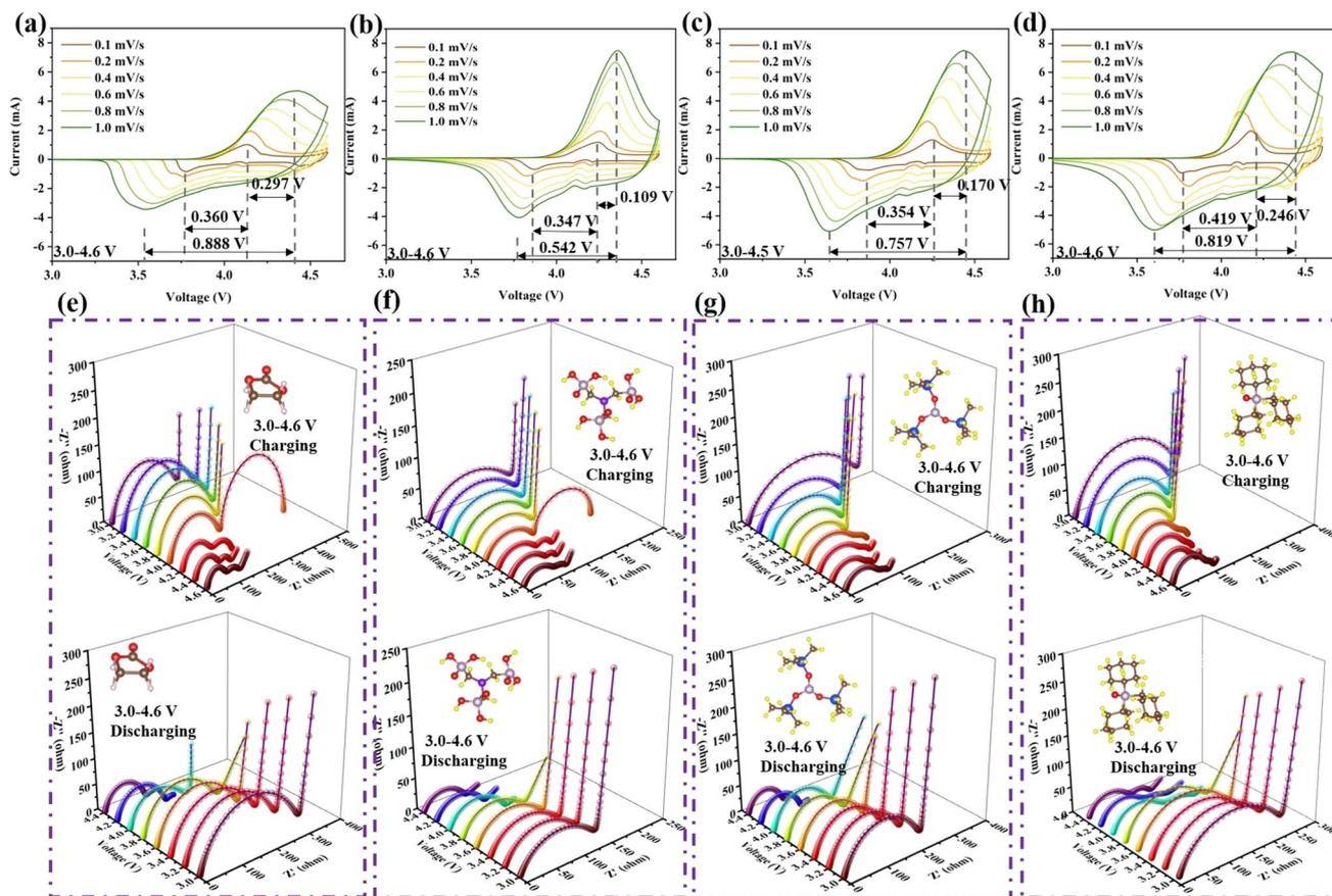
Fig. 2 (a–d) Cyclic voltammograms at different scanning rates from  $0.1 \text{ mV s}^{-1}$  to  $1.0 \text{ mV s}^{-1}$  for the cells with (a) LED, (b) LAED, (c) LTMED, and (d) LTPED. *In situ* EIS testing during the charging and discharging process from 100 kHz to 10 Hz with different electrolytes: (e) LED, (f) LAED, (g) LTMED, and (h) LTPED under 3.0–4.6 V.
