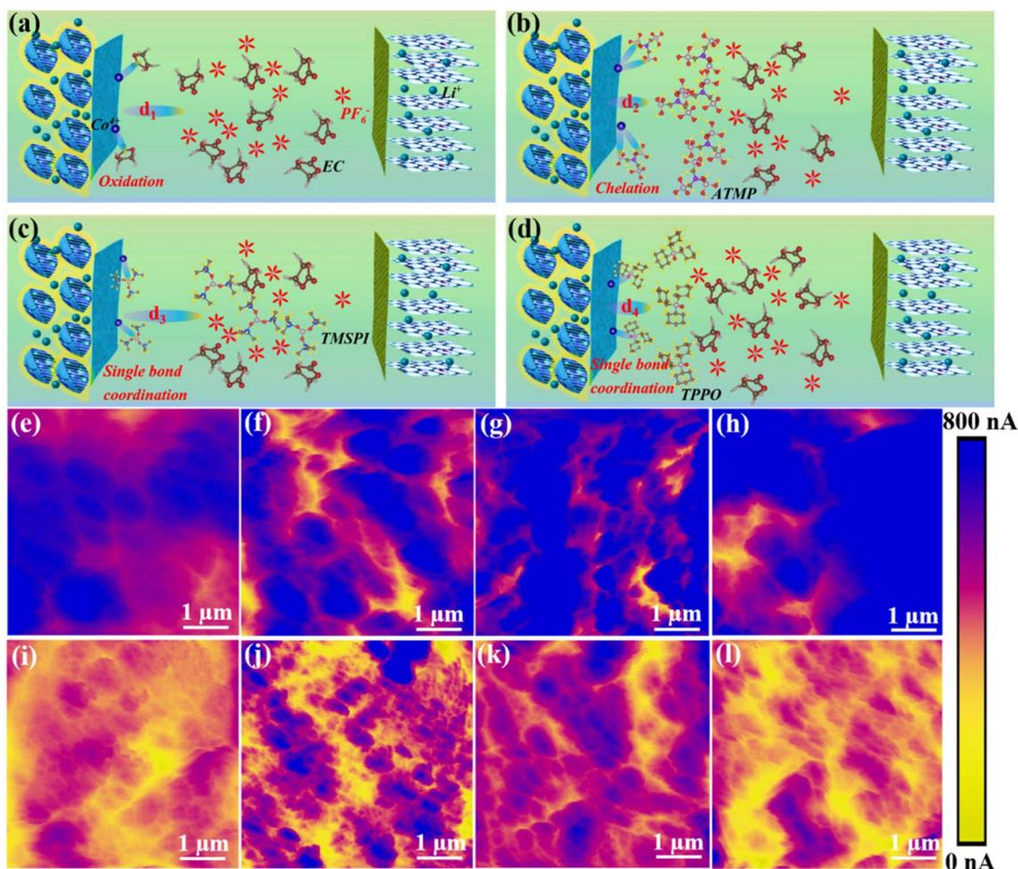
Fig. 4 Interfacial interaction model. (a) EC and cathode, (b) ATMP and cathode, (c) TMSPI and cathode, (d) TPPO and cathode. *Ex situ* c-AFM detection of interface conductivity of cathode after 1 cycle with different electrolytes: (e) LED, (f) LAED, (g) LTMED, and (h) LTPED. The conductivity of the cathode interface after 200 cycles also detected with different electrolytes: (i) LED, (j) LAED, (k) LTMED, and (l) LTPED.
