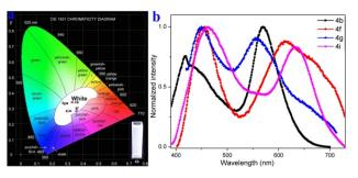
Fig. 1 Fluorescence properties. (a) Commission Internationale de l'Eclairage (CIE) coordinates of 4b (0.33, 0.34), 4f (0.36, 0.28), 4g (0.30, 0.33), and 4i (0.32, 0.28) in CH<sub>2</sub>Cl<sub>2</sub>, respectively. (b) Fluorescence emission spectra of 4b, 4f, 4g, and 4i in CH<sub>2</sub>Cl<sub>2</sub> (concentration: 4b: 0.1  $\mu$ M; 4f: 250  $\mu$ M; 4g: 500  $\mu$ M; 4i: 50  $\mu$ M).
