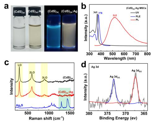
Fig. 1 (a) Photographs of  $(CdS)_{34}$  and  $(CdS)_{34}$ :Ag MSCs under natural and UV light. (b) UV-vis absorption, PL and PLE spectra of  $(CdS)_{34}$ :Ag MSCs. (c) Raman spectra of  $(CdS)_{34}$ :Ag MSCs and Ag<sub>2</sub>S. (d) High-resolution X-ray photoelectron spectra of  $(CdS)_{34}$ :Ag MSCs in the Ag 3d electron binding energy range.
