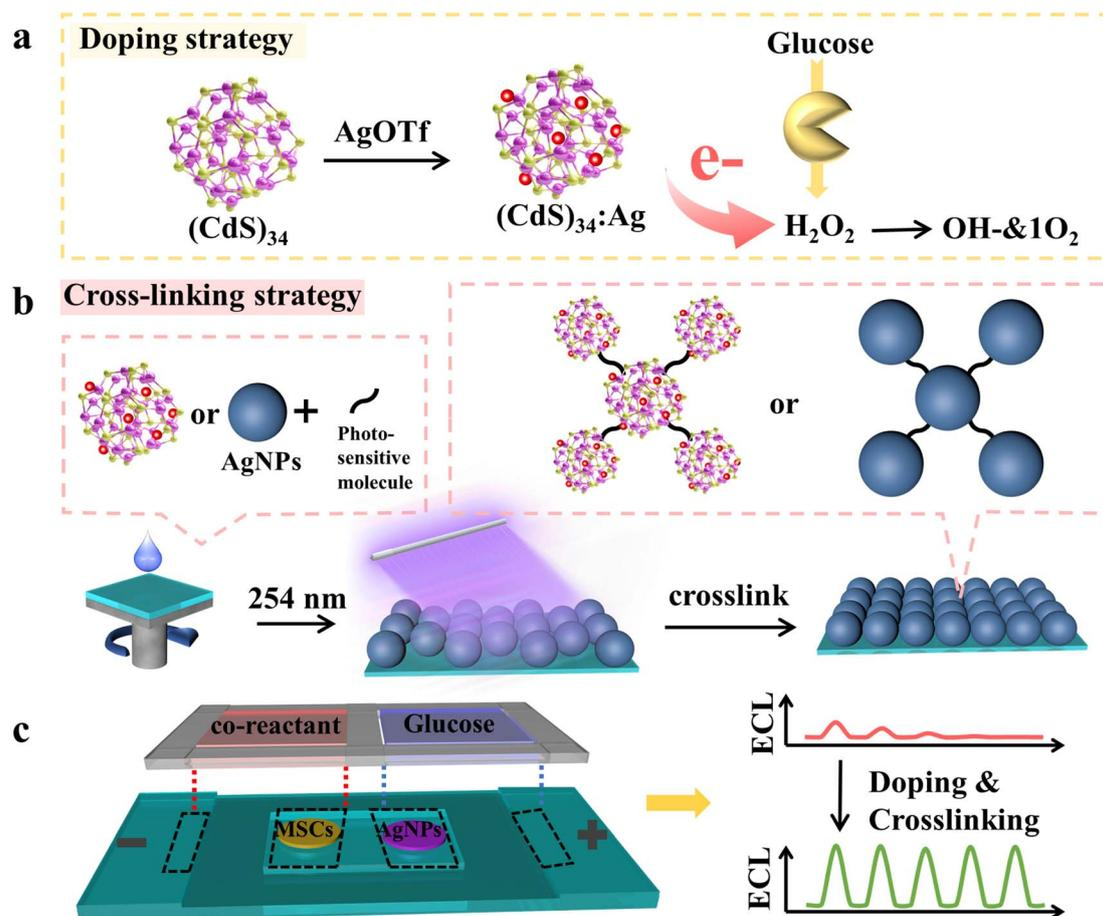
Scheme 1 Schematic illustrations of (a) the doping strategy of  $(\text{CdS})_{34}$  MSCs and the detection principle of glucose. (b) Cross-linking strategy of  $(\text{CdS})_{34}:\text{Ag}$  MSCs and Ag NPs. (c) Construction of the BPE system.
