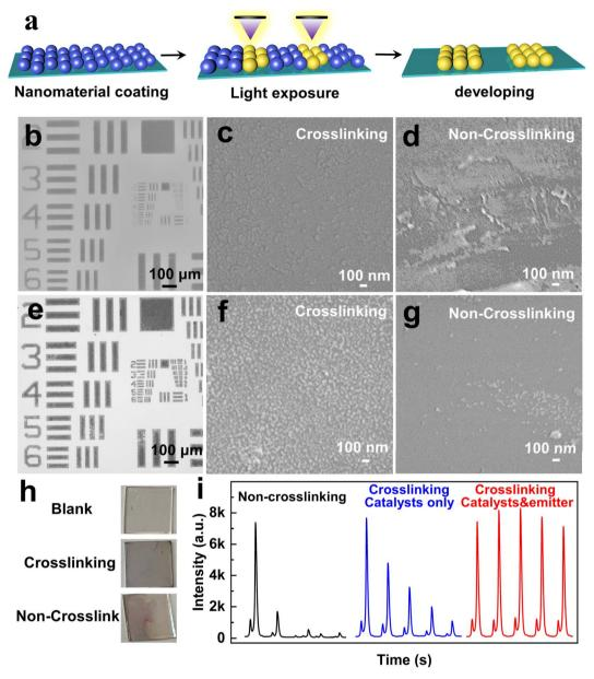
Fig. 3 (a) Outline of the processing steps for lithography by crosslinking. Microscopic imaging of lithography by crosslinking for (b) (CdS)<sub>34</sub>:Ag MSCs and (e) Ag NPs. SEM image of (c) (CdS)<sub>34</sub>:Ag MSCs with and (d) without crosslinking; (f) Ag NPs with and (g) without crosslinking; (h) photo of Ag NPs attached to ITO and (i) ECL intensities of the BPE system with different crosslinking conditions.
