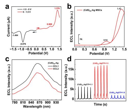
Fig. 2 (a) DPV curve of (CdS)<sub>34</sub>:Ag MSCs, (b) ECL-E curve of (CdS)<sub>34</sub>:Ag MSCs. (c) ECL spectra of (CdS)<sub>34</sub>:Ag MSCs at different potentials (ECL1 at 0.9 V; ECL2 at 1.4 V). (d) ECL intensity of (CdS)<sub>34</sub>:Ag MSCs with different feeding ratios ((CdS)<sub>34</sub>: AgOTf = 1:1, 1:3 and 1:6).
