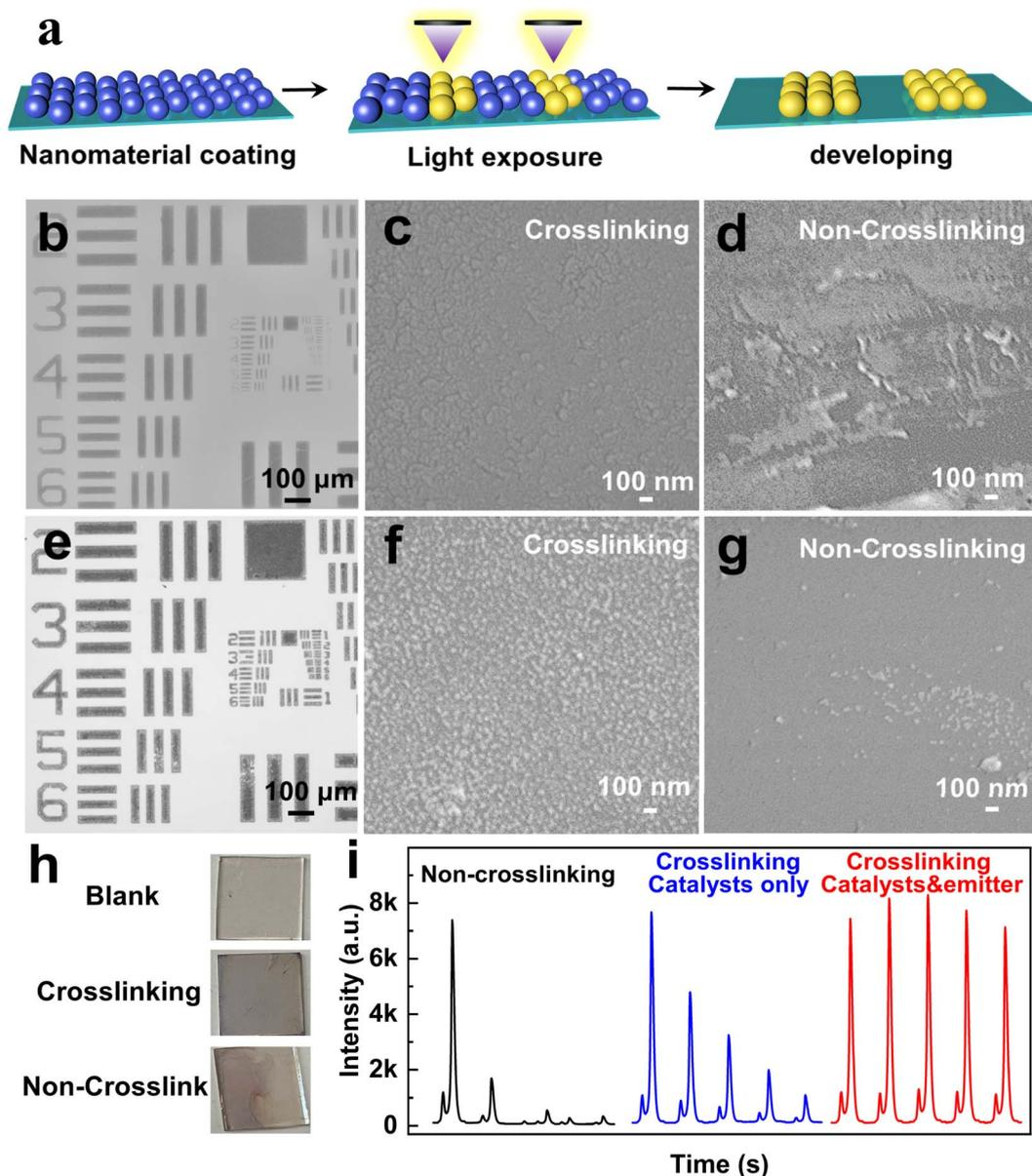
Fig. 3 (a) Outline of the processing steps for lithography by crosslinking. Microscopic imaging of lithography by crosslinking for (b)  $(\text{CdS})_{34}:\text{Ag}$  MSCs and (e) Ag NPs. SEM image of (c)  $(\text{CdS})_{34}:\text{Ag}$  MSCs with and (d) without crosslinking; (f) Ag NPs with and (g) without crosslinking; (h) photo of Ag NPs attached to ITO and (i) ECL intensities of the BPE system with different crosslinking conditions.
