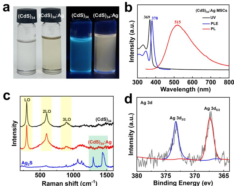
Fig. 1 (a) Photographs of  $(\text{CdS})_{34}$  and  $(\text{CdS})_{34}:\text{Ag}$  MSCs under natural and UV light. (b) UV-vis absorption, PL and PLE spectra of  $(\text{CdS})_{34}:\text{Ag}$  MSCs. (c) Raman spectra of  $(\text{CdS})_{34}$ ,  $(\text{CdS})_{34}:\text{Ag}$  MSCs and  $\text{Ag}_2\text{S}$ . (d) High-resolution X-ray photoelectron spectra of  $(\text{CdS})_{34}:\text{Ag}$  MSCs in the Ag 3d electron binding energy range.
