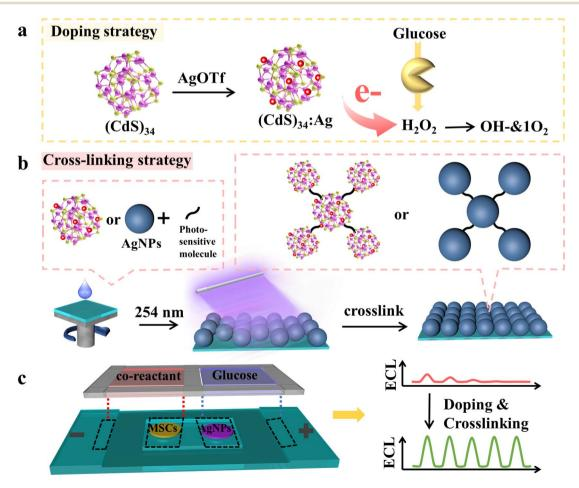
Scheme 1 Schematic illustrations of (a) the doping strategy of  $(CdS)_{34}$  MSCs and the detection principle of glucose. (b) Cross-linking strategy of  $(CdS)_{34}$ :Ag MSCs and Ag NPs. (c) Construction of the BPE system.
