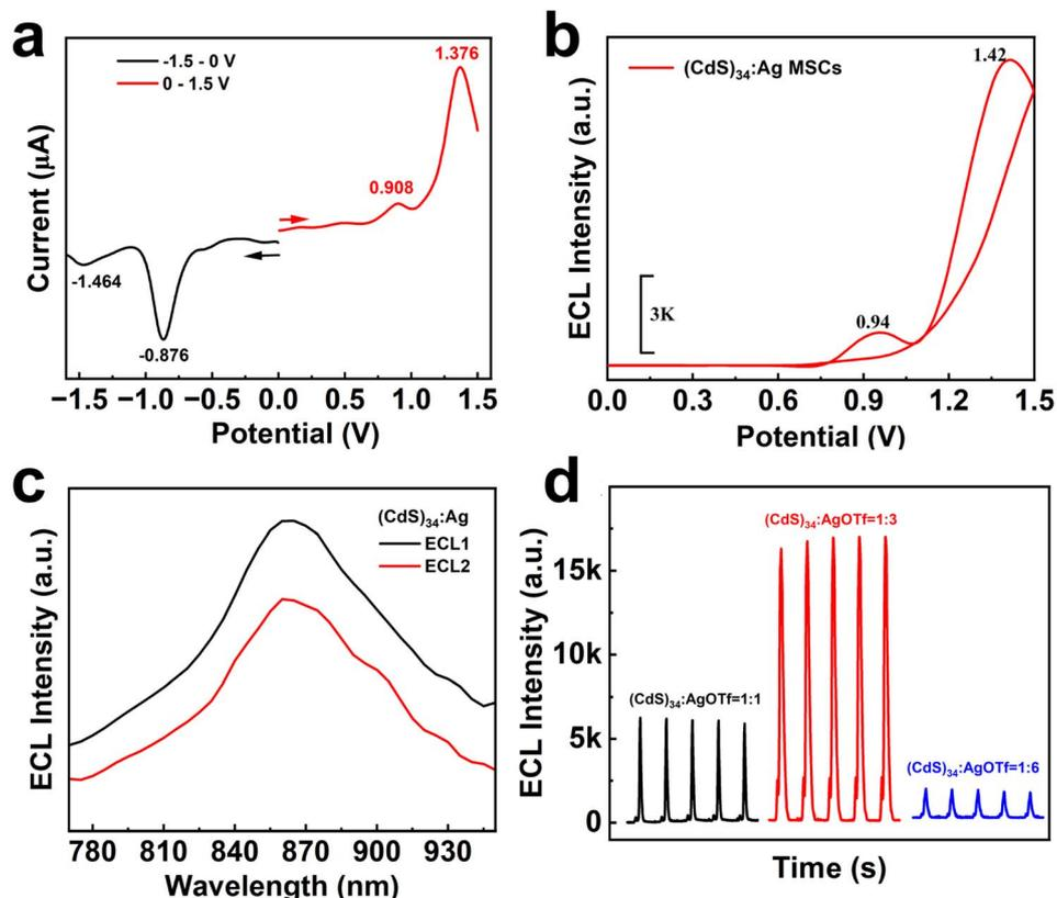
Fig. 2 (a) DPV curve of  $(\text{CdS})_{34}:\text{Ag}$  MSCs, (b) ECL-E curve of  $(\text{CdS})_{34}:\text{Ag}$  MSCs. (c) ECL spectra of  $(\text{CdS})_{34}:\text{Ag}$  MSCs at different potentials (ECL1 at 0.9 V; ECL2 at 1.4 V). (d) ECL intensity of  $(\text{CdS})_{34}:\text{Ag}$  MSCs with different feeding ratios ( $(\text{CdS})_{34}:\text{AgOTf} = 1:1, 1:3$  and  $1:6$ ).
