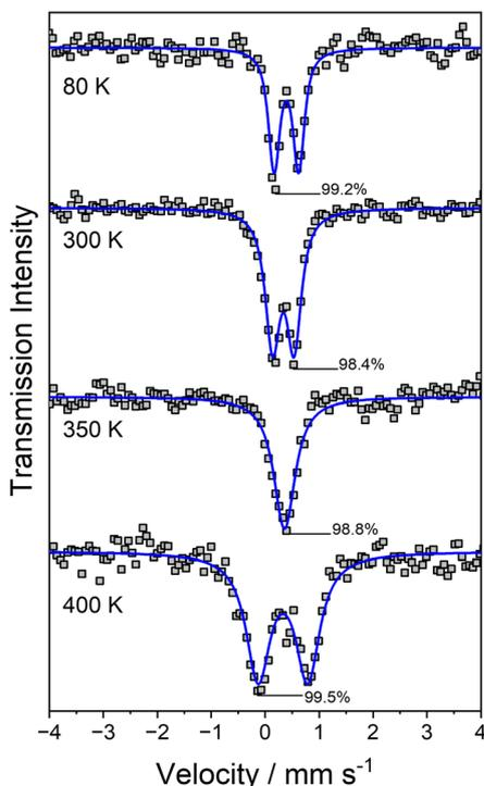
Fig. 5 Variable temperature, zero-field  $^{57}\text{Fe}$  Mössbauer spectra of  $4 \cdot 1.7\text{Pr}_2\text{O}$ . The squares are the raw data, and the solid lines are the least-square Lorentzian fits presented in Table 3.
