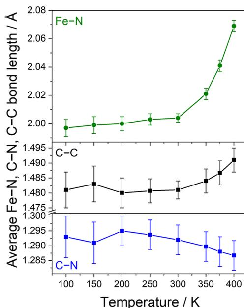
**Fig. 3** Temperature dependence of the average Fe-N bond distances (top) and C-C and C-N bond distances of the Ph-BIAN ligands (bottom) for **4**·2<sup>i</sup>Pr<sub>2</sub>O.
