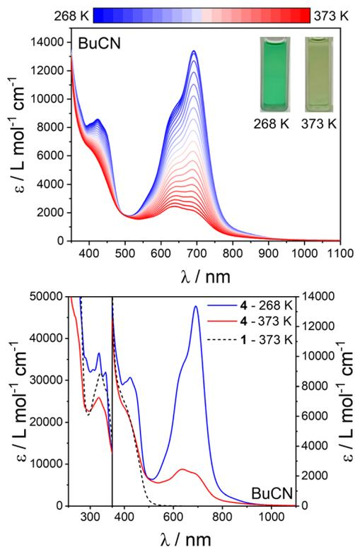
Fig. 9 Top: variable temperature UV-vis absorption spectra of **4** in BuCN between 268 (blue) and 373 K (red) in 5 K increments. Bottom: comparison of the UV-vis spectra of **4** in BuCN at 268 (blue) and 373 K (red) with **1** in BuCN at 373 K.
