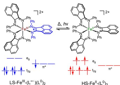
Scheme 1 Valence tautomeric equilibrium  $\text{LS-Fe}^{\text{III}}\text{-(L}^{\cdot-}\text{)}(\text{L}^0)_2 \rightleftharpoons \text{HS-Fe}^{\text{II}}\text{-(L}^0)_3$  displayed by **4** in the solid- and solution-state.
