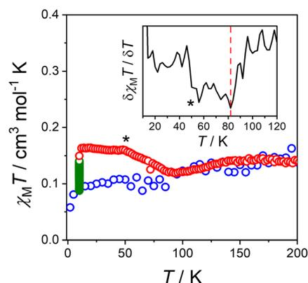
Fig. 7 Plot of  $\chi_M T$  vs.  $T$  for  $4 \cdot 1.7^1\text{Pr}_2\text{O}$  upon cooling (blue circles) response with irradiation with 420 nm for 12 hours at 10 K (green circles), and subsequent warming scan after the light is switched off (red circles). Inset figure shows  $\delta\chi_M T / \delta T$  vs.  $T$ , with  $T(\text{photoirradiation})$  indicated by the red line (82 K). \* Bump due to molecular oxygen.
